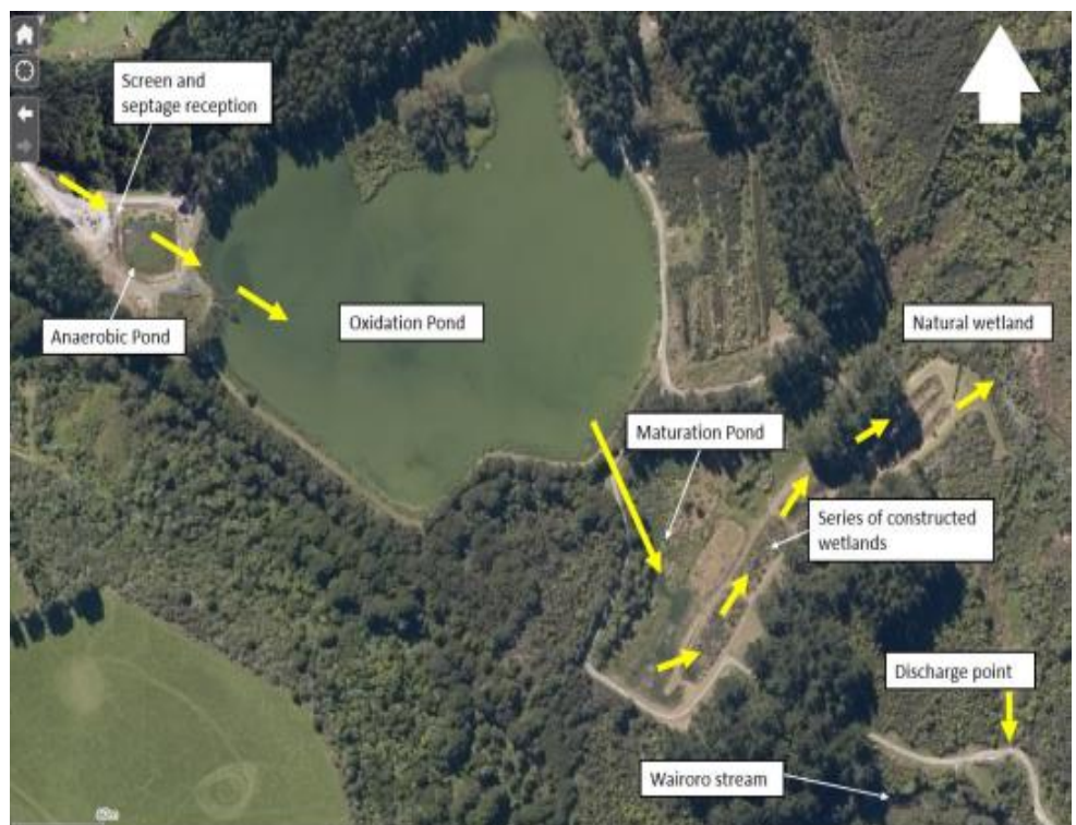
Kaikohe WWTP detailed process of effluent treatment onsite, Cumber Road, Kaikohe. Image taken from WDC GIS Maps 2021.
