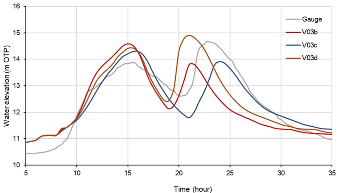
FIGURE 9-6 COMPARISON OF MODELLED AND GAUGED WATER LEVELS FOR TARAWHATAROA AT PURIRI PLACE
