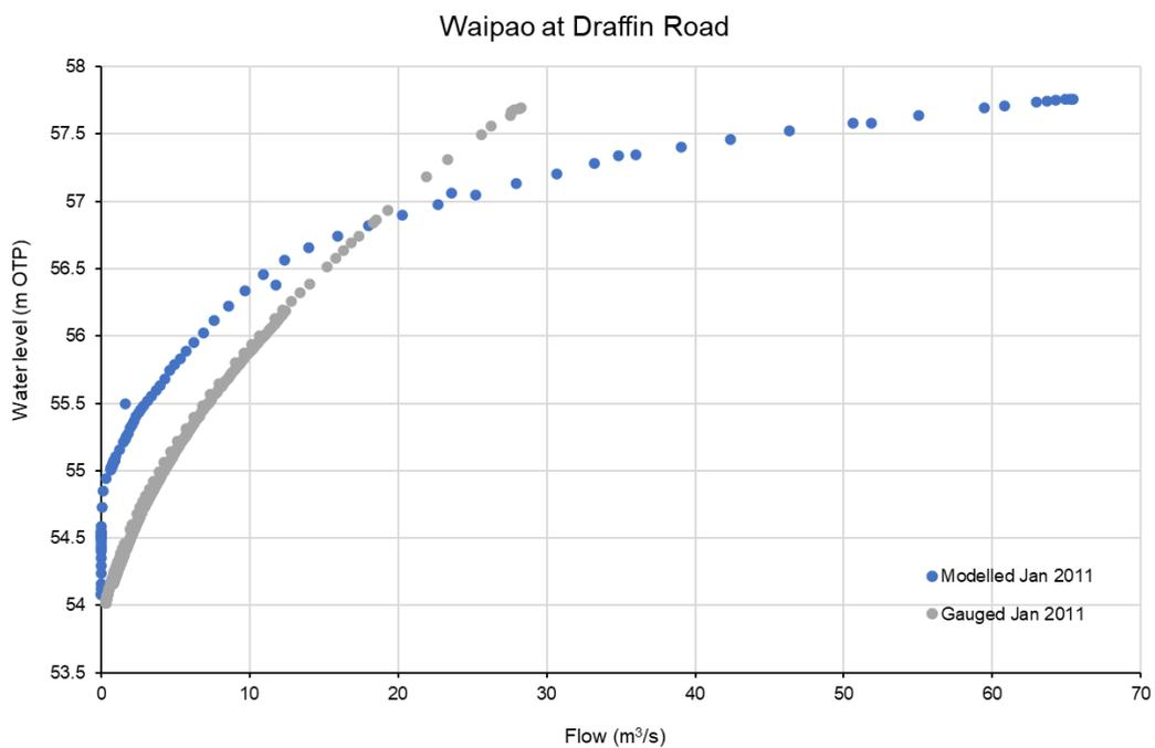
FIGURE 8-17 MODELLED AND GAUGED RATING CURVE COMPARISON AT DRAFFIN RD GAUGE
