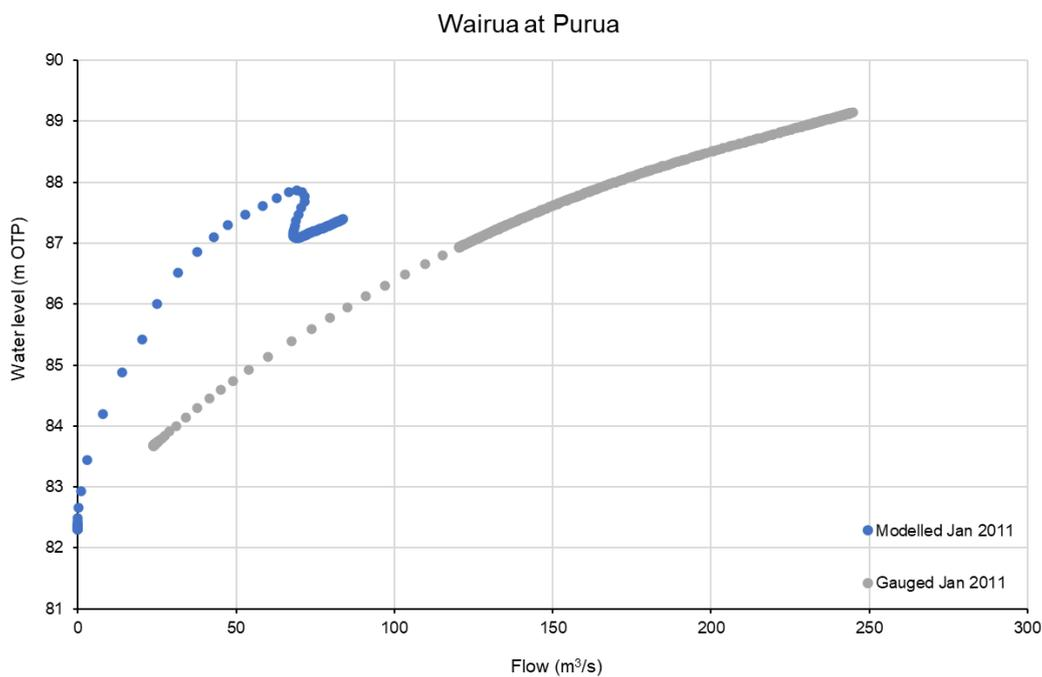
FIGURE 8-15 MODELLED AND GAUGED RATING CURVE COMPARISON AT PURUA GAUGE
