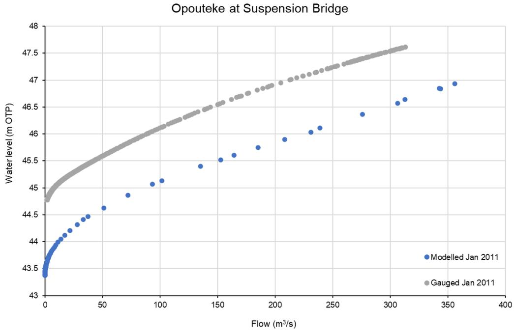
**FIGURE 7-17 MODELLED AND GAUGED RATING CURVE COMPARISON AT SUSPENSION BRIDGE**
