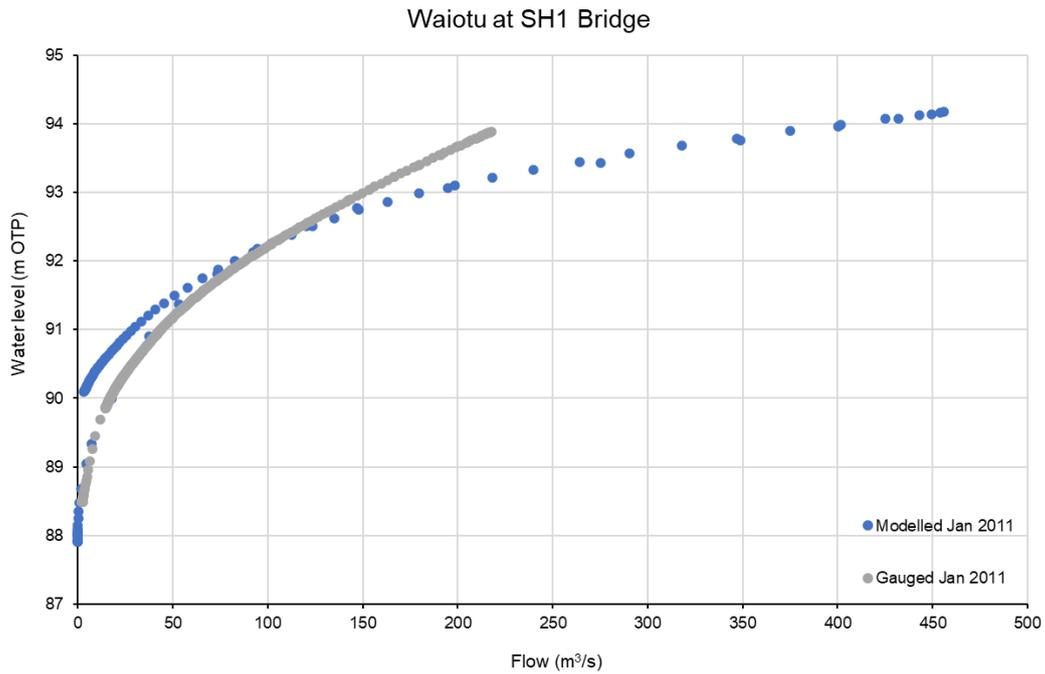
**FIGURE 8-12 MODELLED AND GAUGED RATING CURVE COMPARISON AT S.H. 1 BRIDGE GAUGE**
