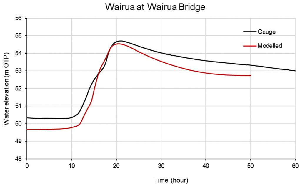
FIGURE 8-11 MODELLED AND GAUGED WATER LEVEL COMPARISON AT WAIRUA BRIDGE GAUGE – M14
