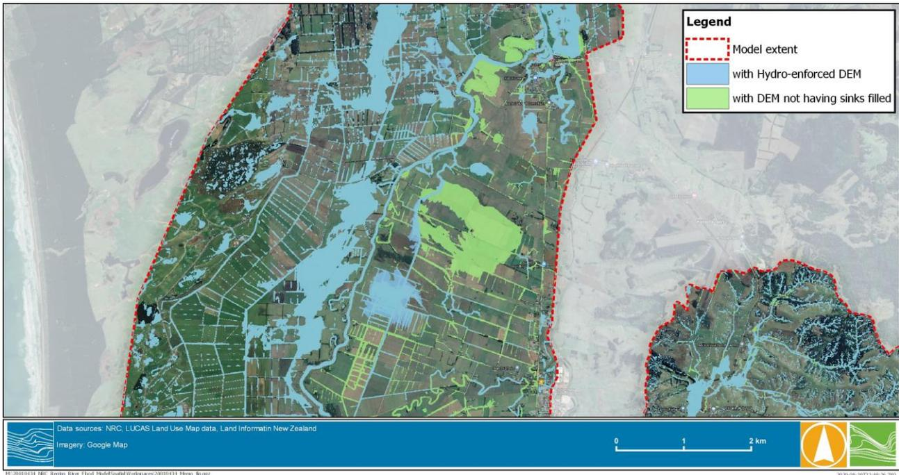
**FIGURE 3-6 MISSING OF FLOODING AREAS USING HYDRO-ENFORCED DEM**
