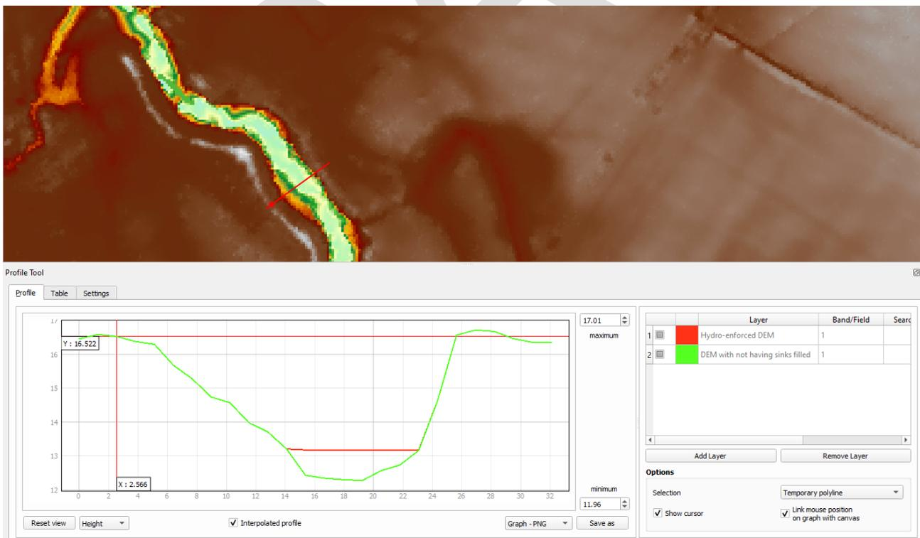
**FIGURE 3-5 DRAINAGE TOPOGRAPHY IN HYDRO-ENFORCED DEM**
