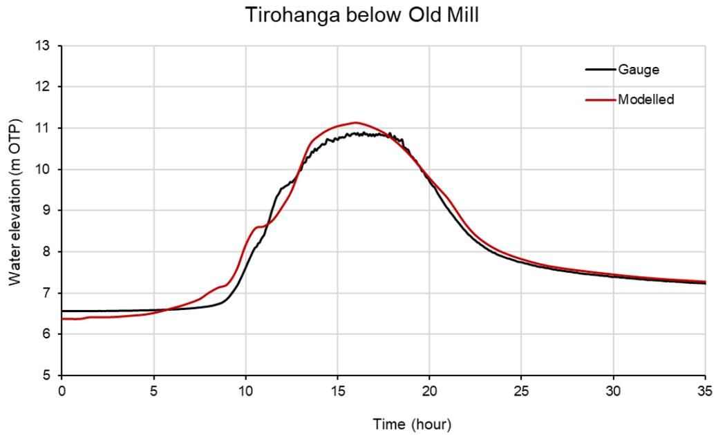
FIGURE 5-10 MODELLED AND GAUGED WATER LEVELS AT TIROHANGA RIVER BELOW OLD MILL
