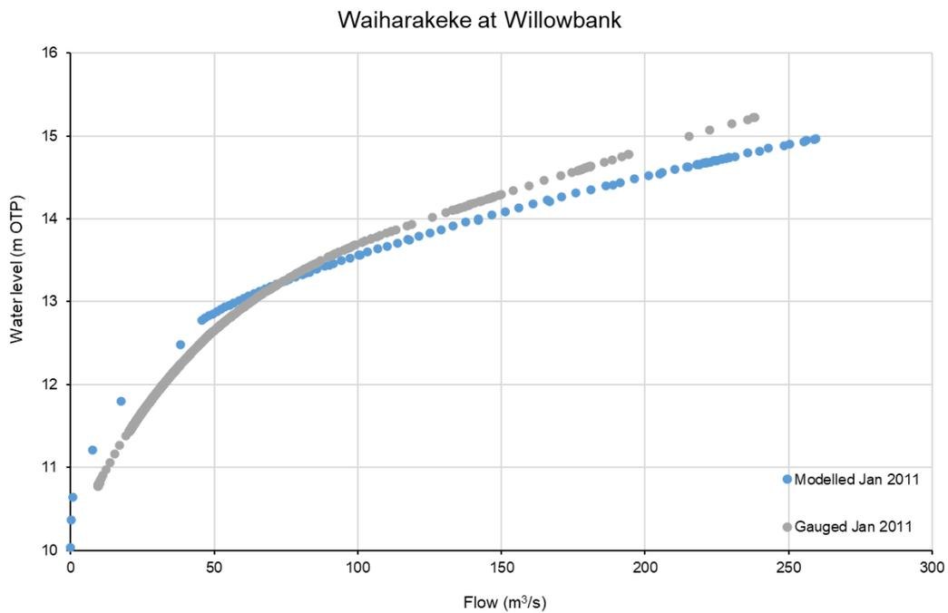
FIGURE 5-11 MODELLED AND GAUGED RATING CURVE COMPARISON AT WILLOWBANK GAUGE
