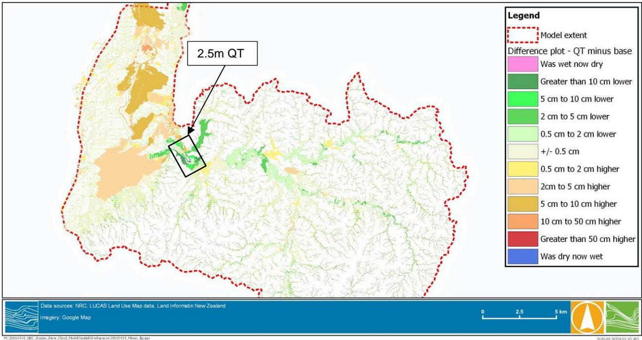
**FIGURE 3-3 FLOOD LEVEL DIFFERENCE PLOT (QUADTREE AND BASE SCENARIO)**
