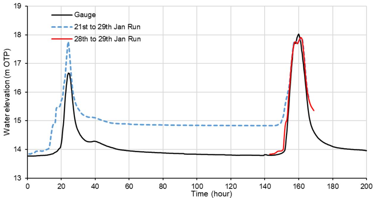
FIGURE 9-12 MODELLED WATER LEVEL HYDROGRAPHS FROM 21<sup>ST</sup> TO 29<sup>TH</sup> JANUARY RAINFALL – M07
