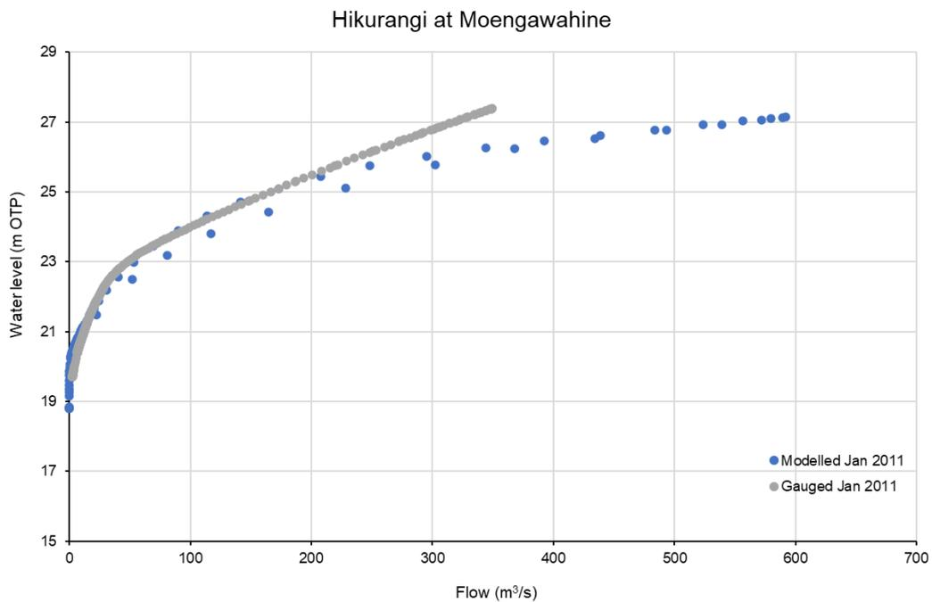
**FIGURE 7-18 MODELLED AND GAUGED RATING CURVE COMPARISON AT MOENGAWAHINE**
