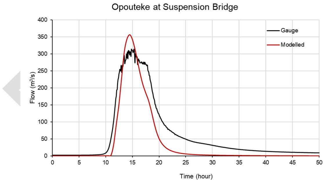
FIGURE 7-8 MODELLED AND GAUGED HYDROGRAPH COMPARISON AT SUSPENSION BRIDGE GAUGE – M13
