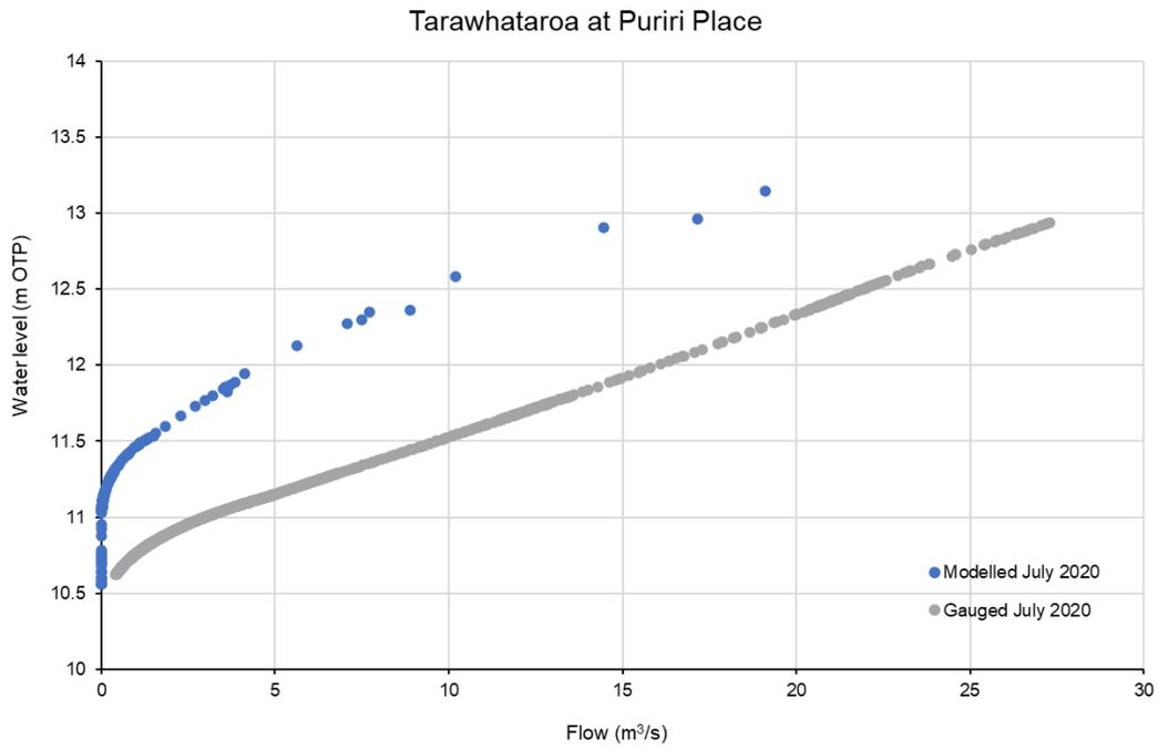
**FIGURE 4-14 MODELLED AND GAUGED RATING CURVE COMPARISON AT PURIRI PLACE**
