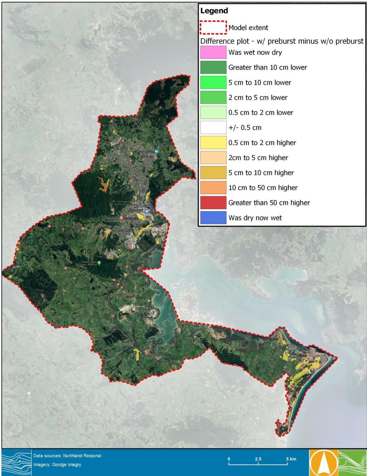
**FIGURE 9-8 DIFFERENCE PLOT OF PREBURST SENSITIVITY TEST IN WHANGAREI CATCHMENT**
