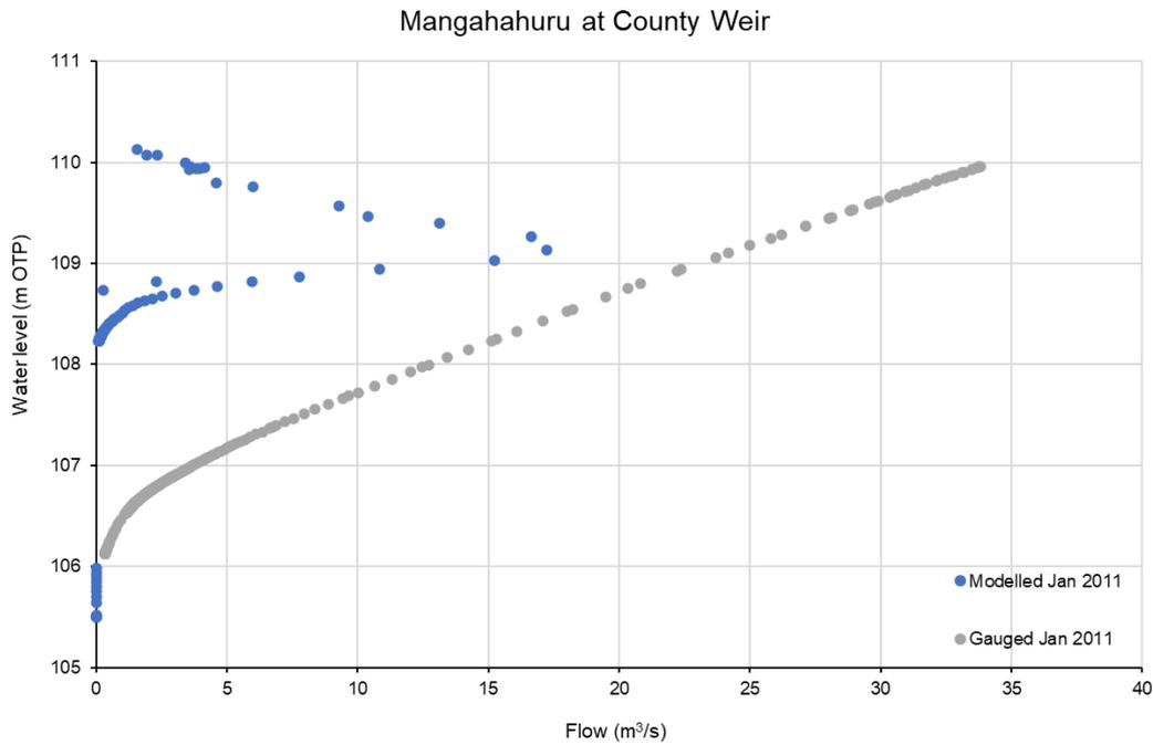
FIGURE 8-14 MODELLED AND GAUGED RATING CURVE COMPARISON AT COUNTY WEIR GAUGE
