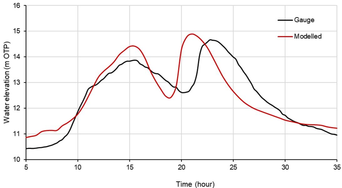
FIGURE 15-7 MODELLED AND GAUGED WATER LEVELS AT TARAWHATORA RIVER AT SCHOOL CUT – 2011 FLOOD EVENT
