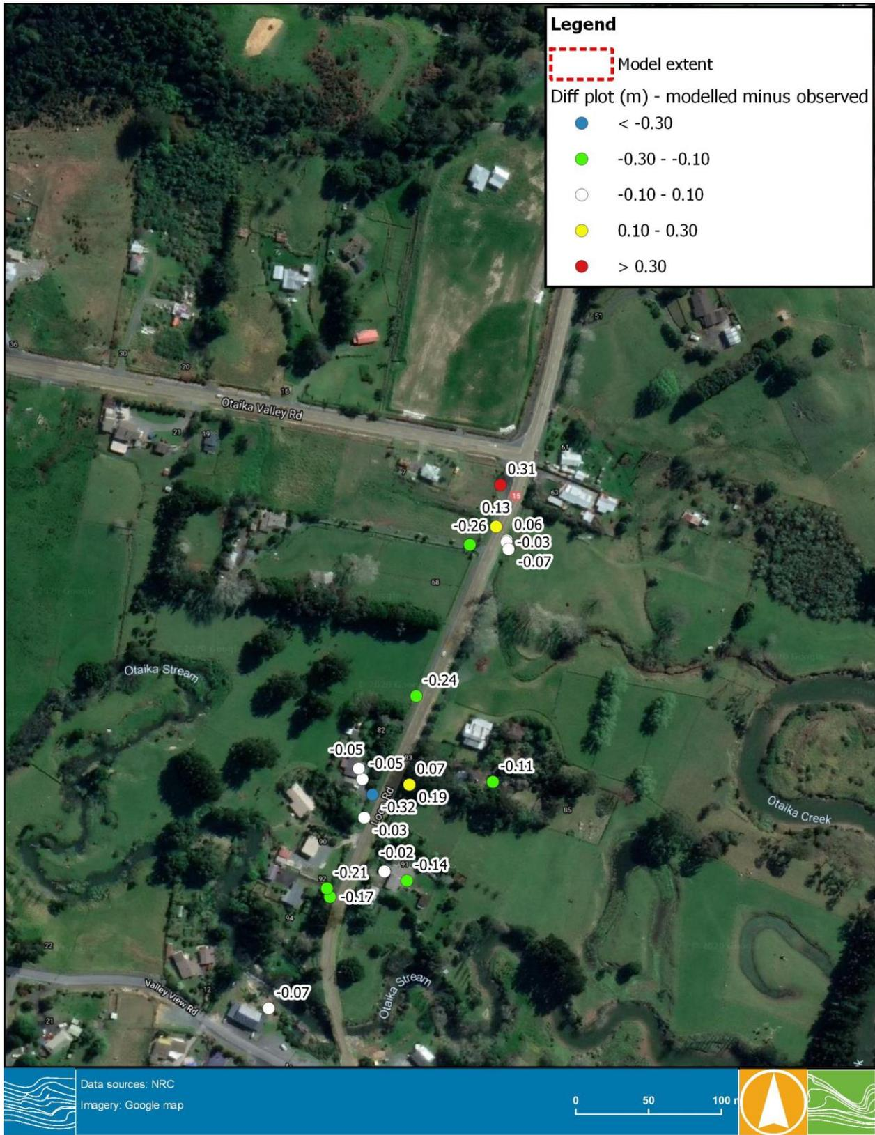
**FIGURE 6-21 COMPARISON BETWEEN MODELLED FLOOD LEVEL AND SURVEY FLOOD LEVEL – JANUARY 2011 EVENT (EAST OF OTAIKA VALLEY RD)**
