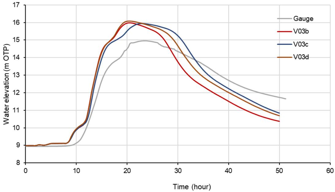
FIGURE 9-5 COMPARISON OF MODELLED AND GAUGED WATER LEVELS FOR AWANUI RIVER AT SCHOOL CUT
