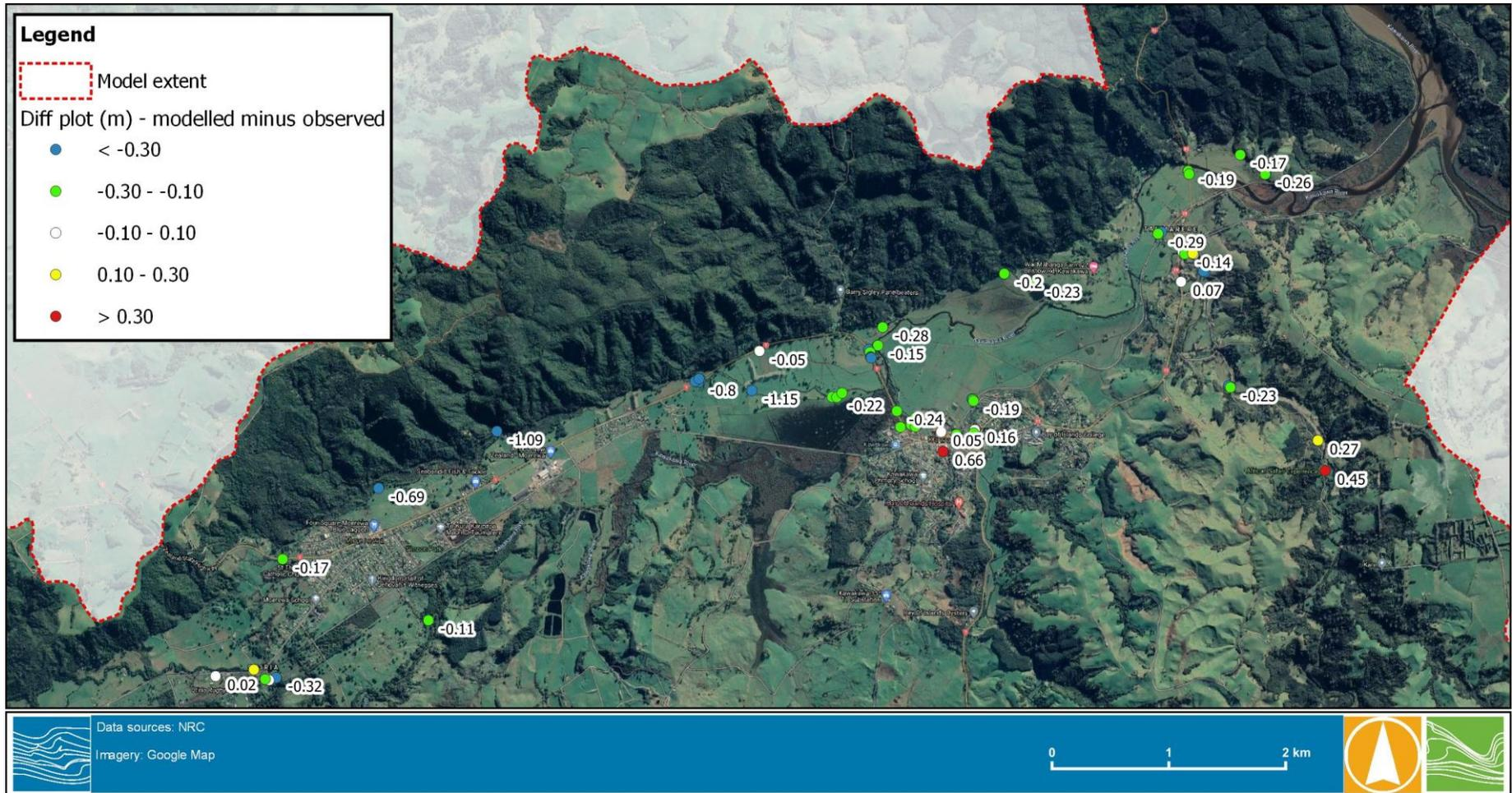
**FIGURE 5-13 COMPARISON BETWEEN MODELLED FLOOD LEVEL AND SURVEY FLOOD LEVEL – JANUARY 2011 EVENT (LOWER KAWAKAWA CATCHMENT)**
