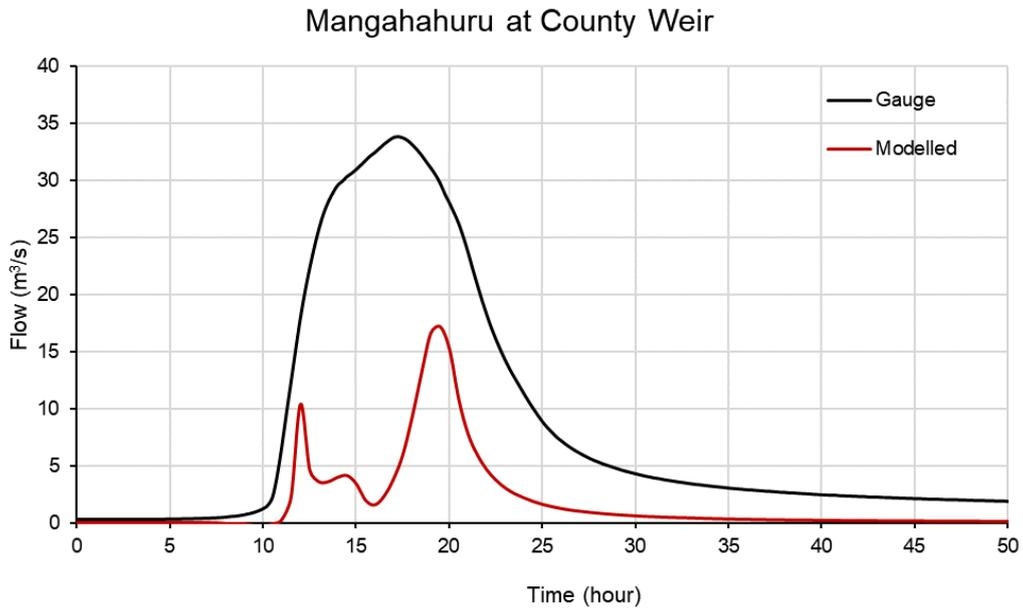
**FIGURE 8-21 MODELLED AND GAUGED HYDROGRAPHS COMPARISON AT COUNTY WEIR GAUGE**
