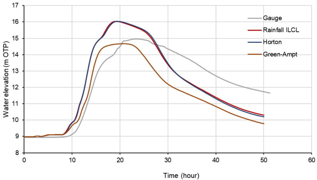
FIGURE 9-2 WATER LEVEL COMPARISON OF DIFFERENT LOSS METHODS – AWANUI RIVER AT SCHOOL CUT
