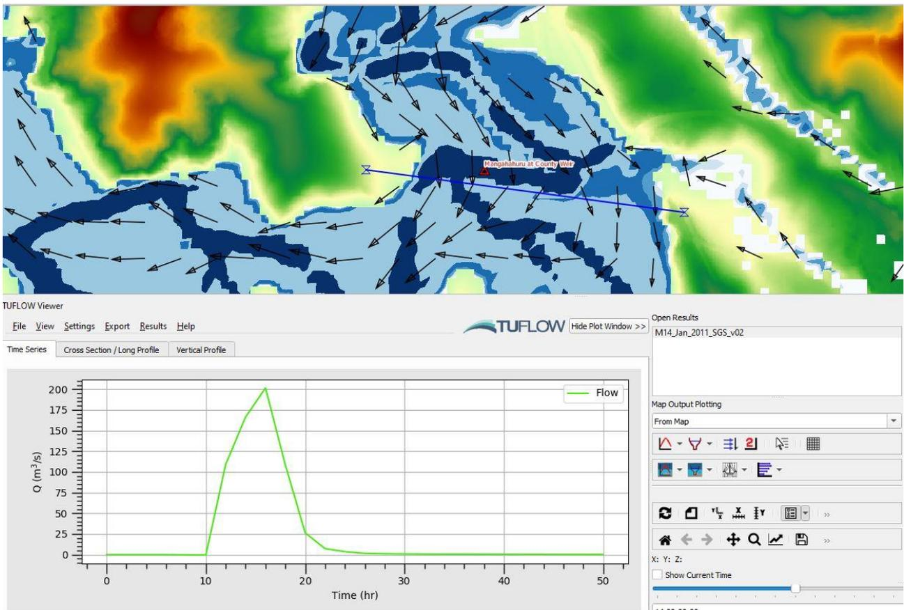
**FIGURE 8-23 PEAK FLOOD FLOW DIRECTION AT COUNTY WEIR GAUGE**
