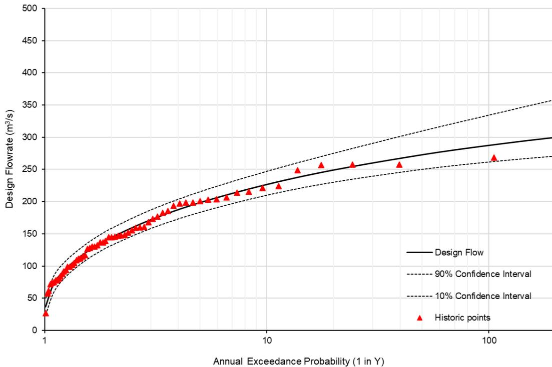
**FIGURE 13-1 EXAMPLE OF FLOOD FREQUENCY CURVE OF LOG PEARSON III - AWANUI AT SCHOOL CUT STREAMFLOW GAUGING STATION**
