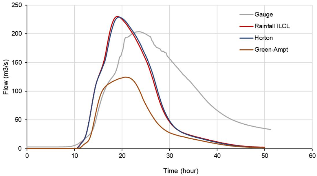
FIGURE 9-1 FLOW COMPARISON OF DIFFERENT LOSS METHODS – AWANUI RIVER AT SCHOOL CUT
