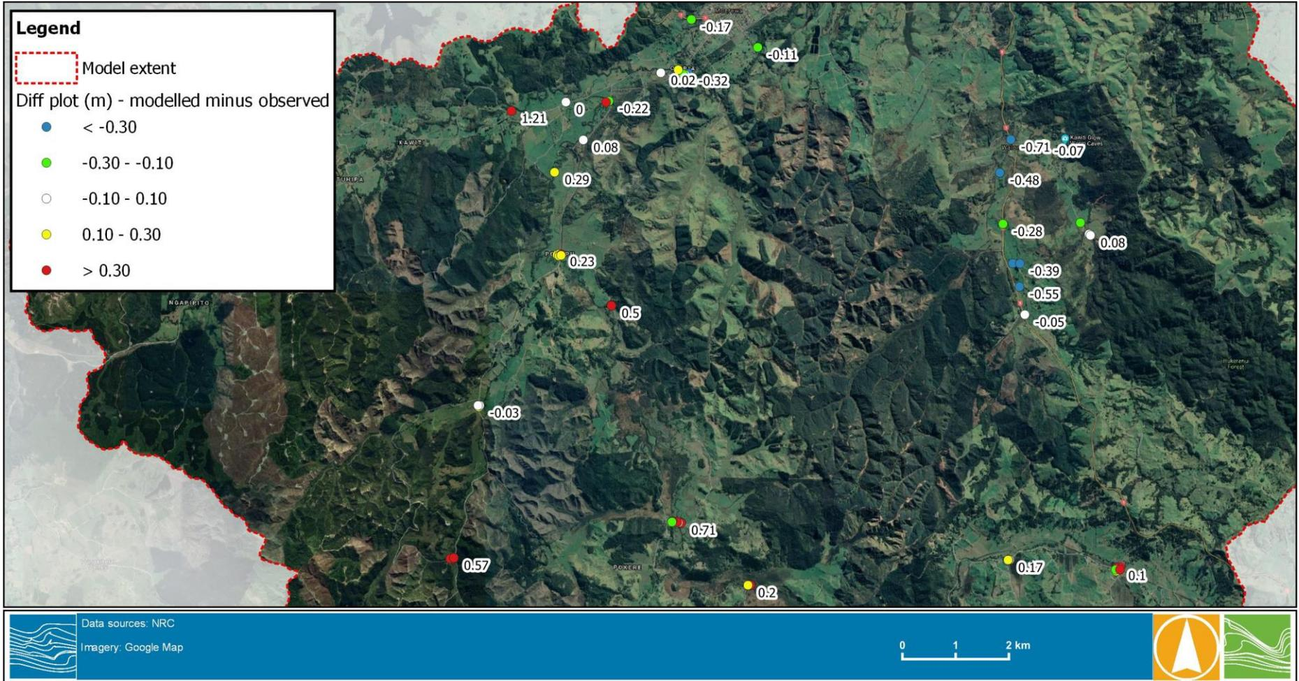
**FIGURE 5-14 COMPARISON BETWEEN MODELLED FLOOD LEVEL AND SURVEY FLOOD LEVEL – JANUARY 2011 EVENT (UPPER KAWAKAWA CATCHMENT)**
