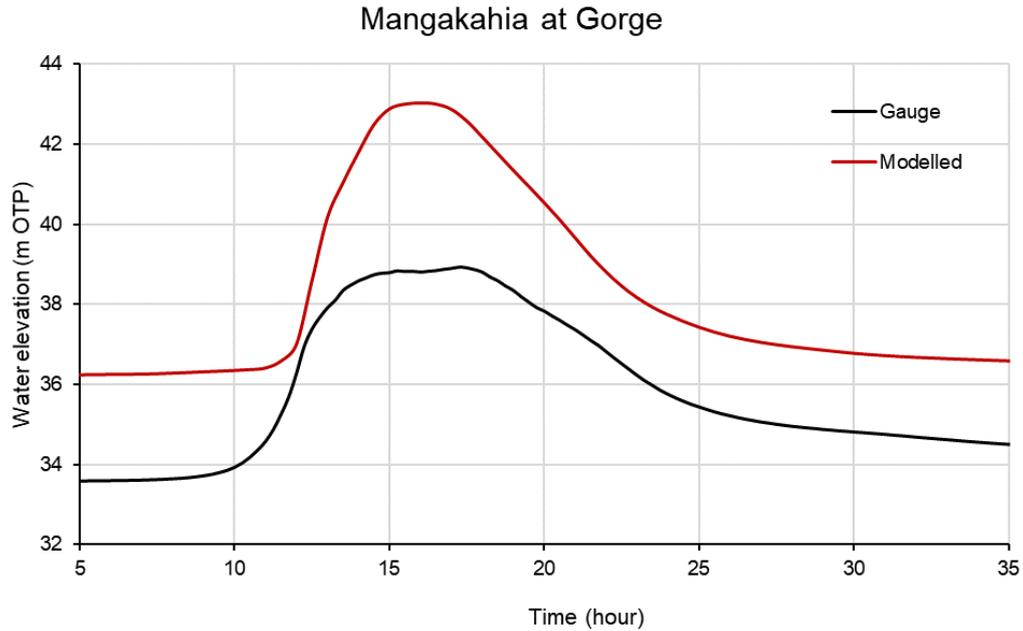
FIGURE 7-7 MODELLED AND GAUGED WATER LEVEL COMPARISON AT GORGE GAUGE – M13
