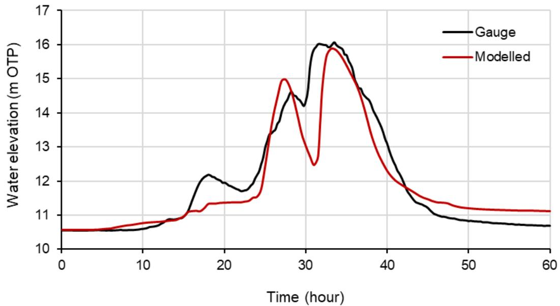
FIGURE 15-11 MODELLED AND GAUGED WATER LEVELS AT TARAWHATORA RIVER AT SCHOOL CUT - JULY 2007 EVENT
