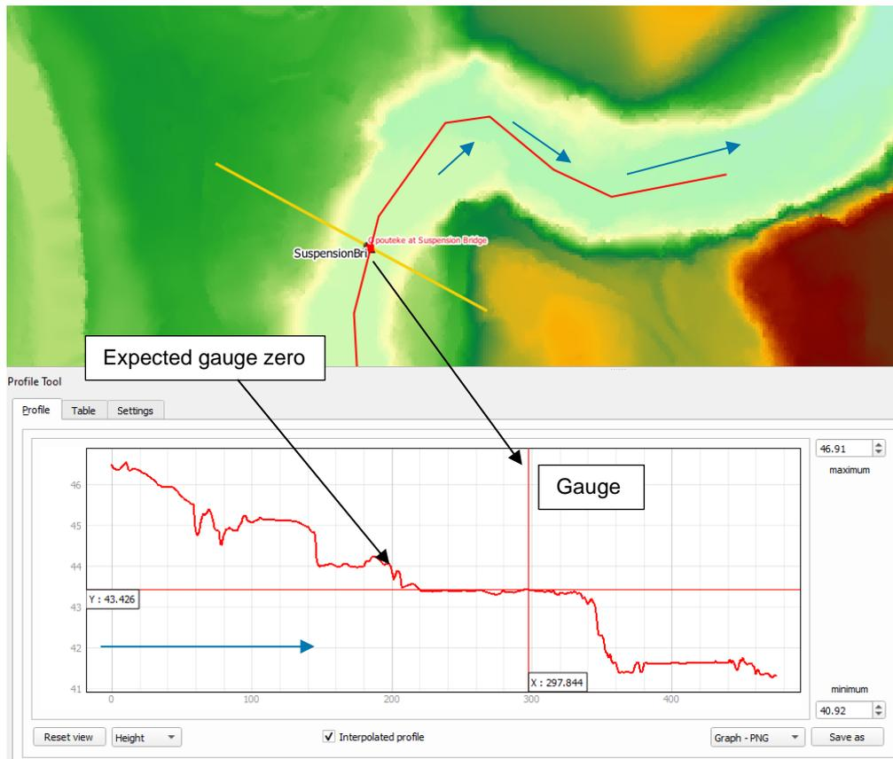
**FIGURE 7-15 LONG SECTION PROFILE UP AND DOWNSTREAM OF SUSPENSION BRIDGE GAUGE**
