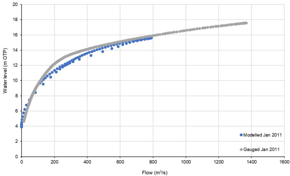
**FIGURE 7-19 MODELLED AND GAUGED RATING CURVE COMPARISON AT TITOKI BRIDGE**
