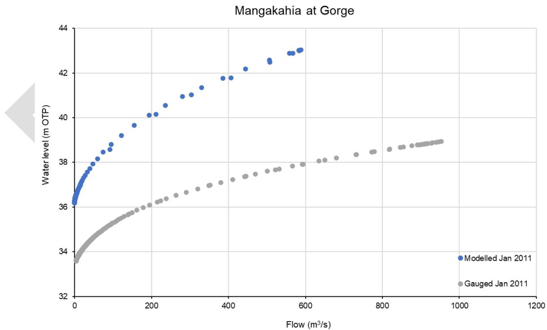
**FIGURE 7-16 MODELLED AND GAUGED RATING CURVE COMPARISON AT GORGE GAUGE**
