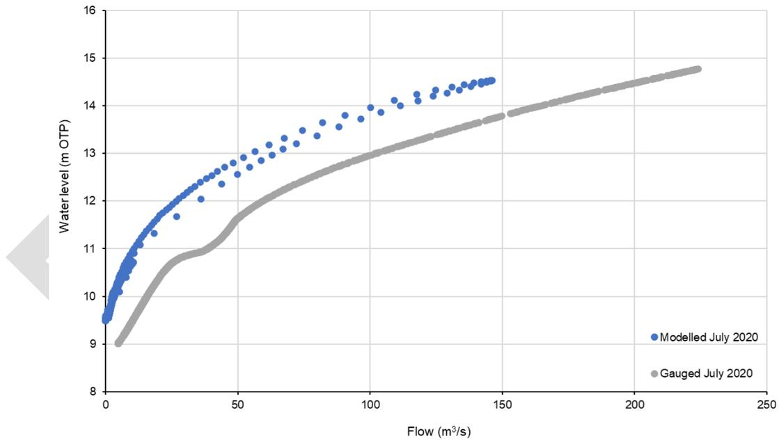
FIGURE 4-13 MODELLED AND GAUGED RATING CURVE COMPARISON AT SCHOOL CUT
