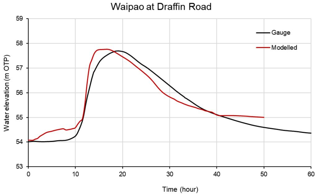
FIGURE 8-10 MODELLED AND GAUGED WATER LEVEL COMPARISON AT DRAFFIN RD GAUGE – M14
