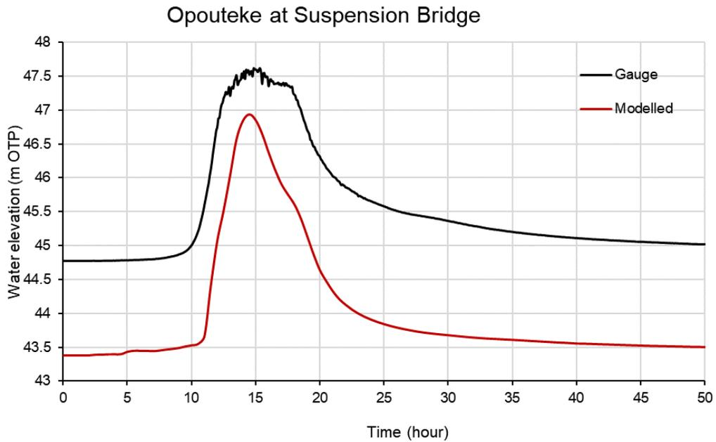
FIGURE 7-9 MODELLED AND GAUGED WATER LEVEL COMPARISON AT SUSPENSION BRIDGE GAUGE – M13
