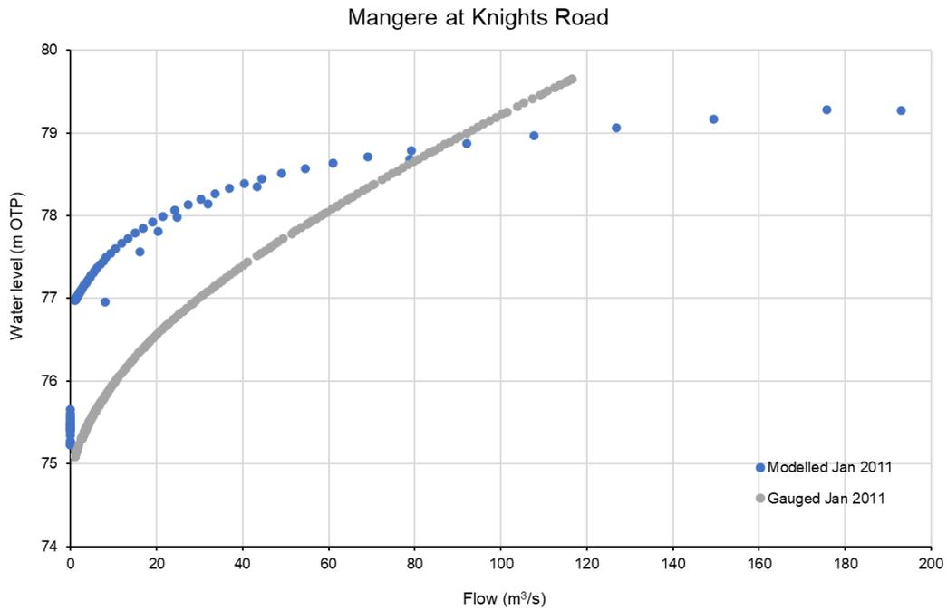
FIGURE 8-16 MODELLED AND GAUGED RATING CURVE COMPARISON AT KNIGHT RD GAUGE
