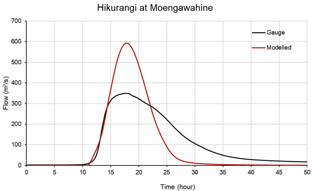
FIGURE 7-10 MODELLED AND GAUGED HYDROGRAPH COMPARISON AT MOENGAWAHINE GAUGE – M13
