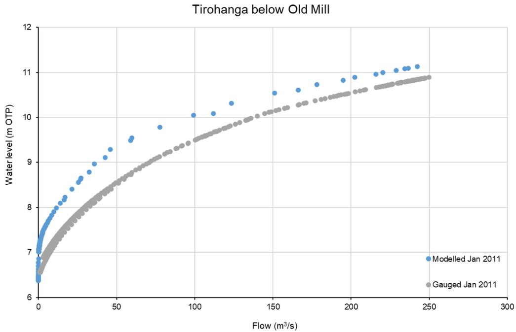
**FIGURE 5-12 MODELLED AND GAUGED RATING CURVE COMPARISON AT OLD MILL GAUGE**
