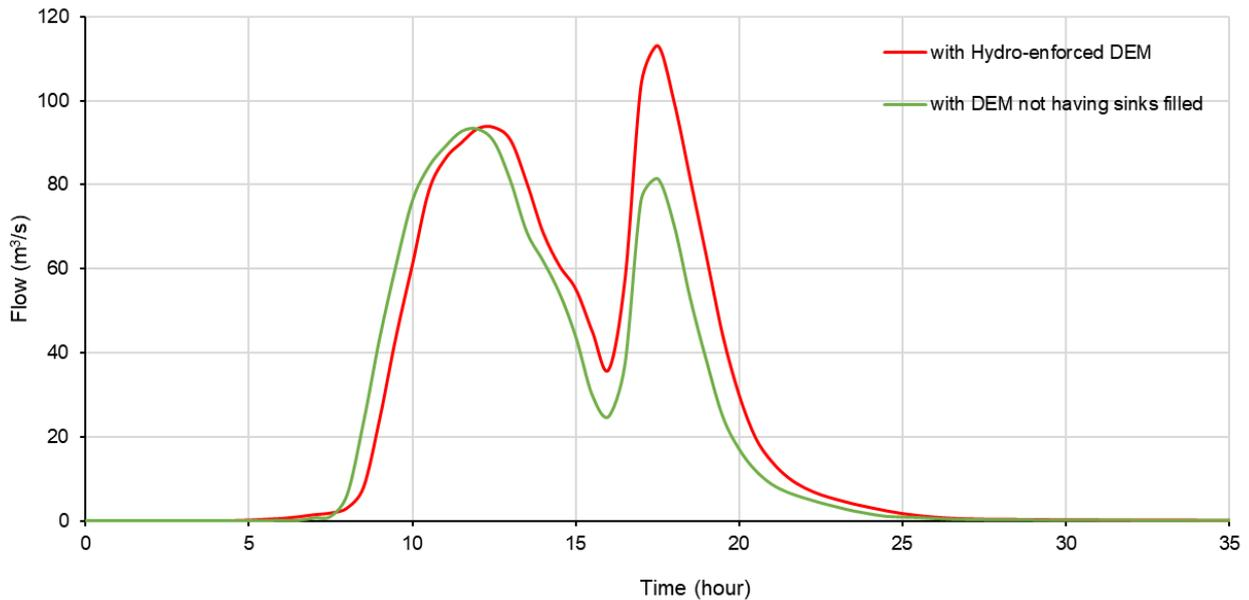
**FIGURE 3-7 PRELIMINARY MODELLED HYDROGRAPH – TARAWHATAROA RIVER AT PURIRI PLACE**
