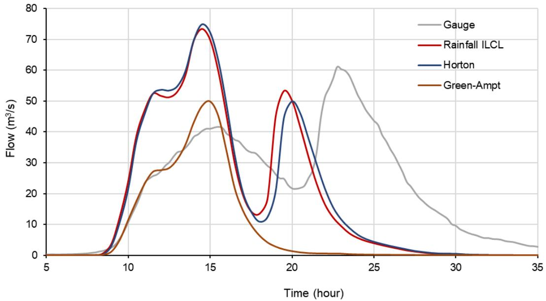
**FIGURE 9-3 FLOW COMPARISON OF DIFFERENT LOSS METHODS – TARAWHATAROA RIVER AT PURIRI PLACE**
