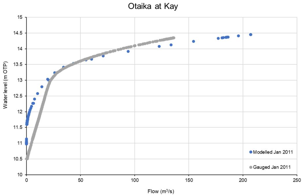
**FIGURE 6-18 MODELLED AND GAUGED RATING CURVE COMPARISON AT KAY**
