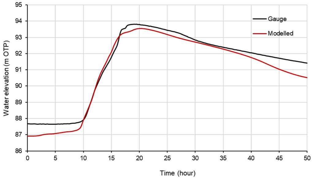
FIGURE 8-6 MODELLED AND GAUGED WATER LEVEL COMPARISON AT CABLEWAY GAUGE – M14
