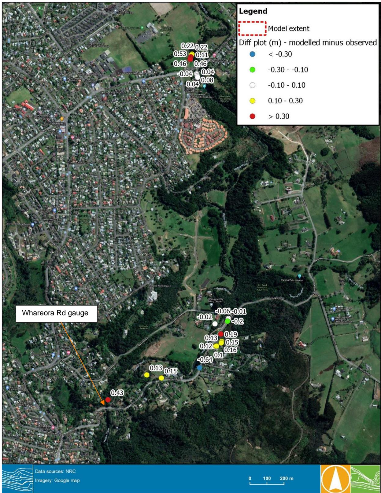
**FIGURE 6-19 COMPARISON BETWEEN MODELLED FLOOD LEVEL AND SURVEY FLOOD LEVEL – JANUARY 2011 EVENT (UPSTREAM OF WHAREORA RD GAUGE)**
