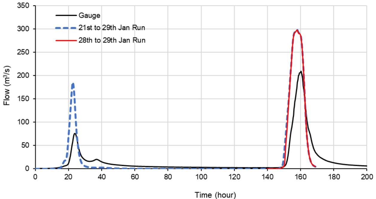
FIGURE 9-10 MODELLED FLOW HYDROGRAPHS FROM 21<sup>ST</sup> TO 29<sup>TH</sup> JANUARY RAINFALL– M06
