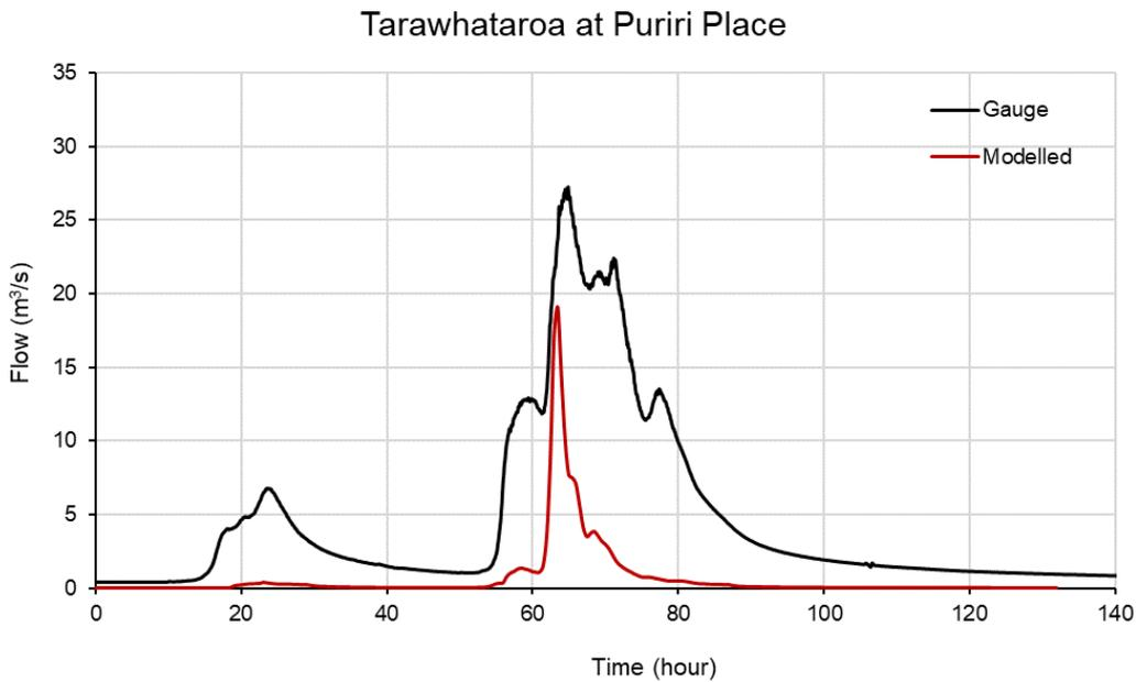
FIGURE 4-11 MODELLED AND GAUGED FLOWS AT TARAWHATAROA RIVER AT PURIRI PLACE – 2020 FLOOD EVENT
