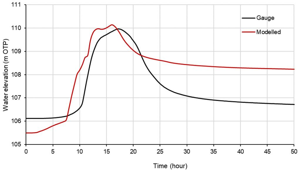
FIGURE 8-7 MODELLED AND GAUGED WATER LEVEL COMPARISON AT COUNTY WEIR GAUGE – M14
