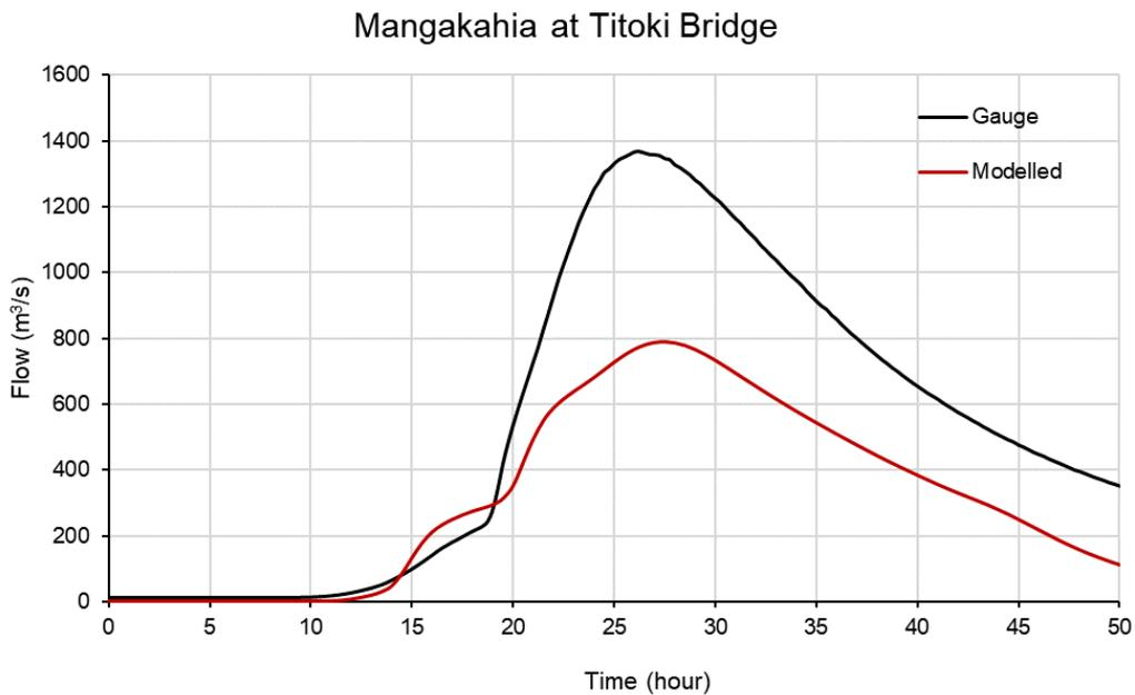
FIGURE 7-12 MODELLED AND GAUGED HYDROGRAPH COMPARISON AT TITOKI GAUGE – M13
