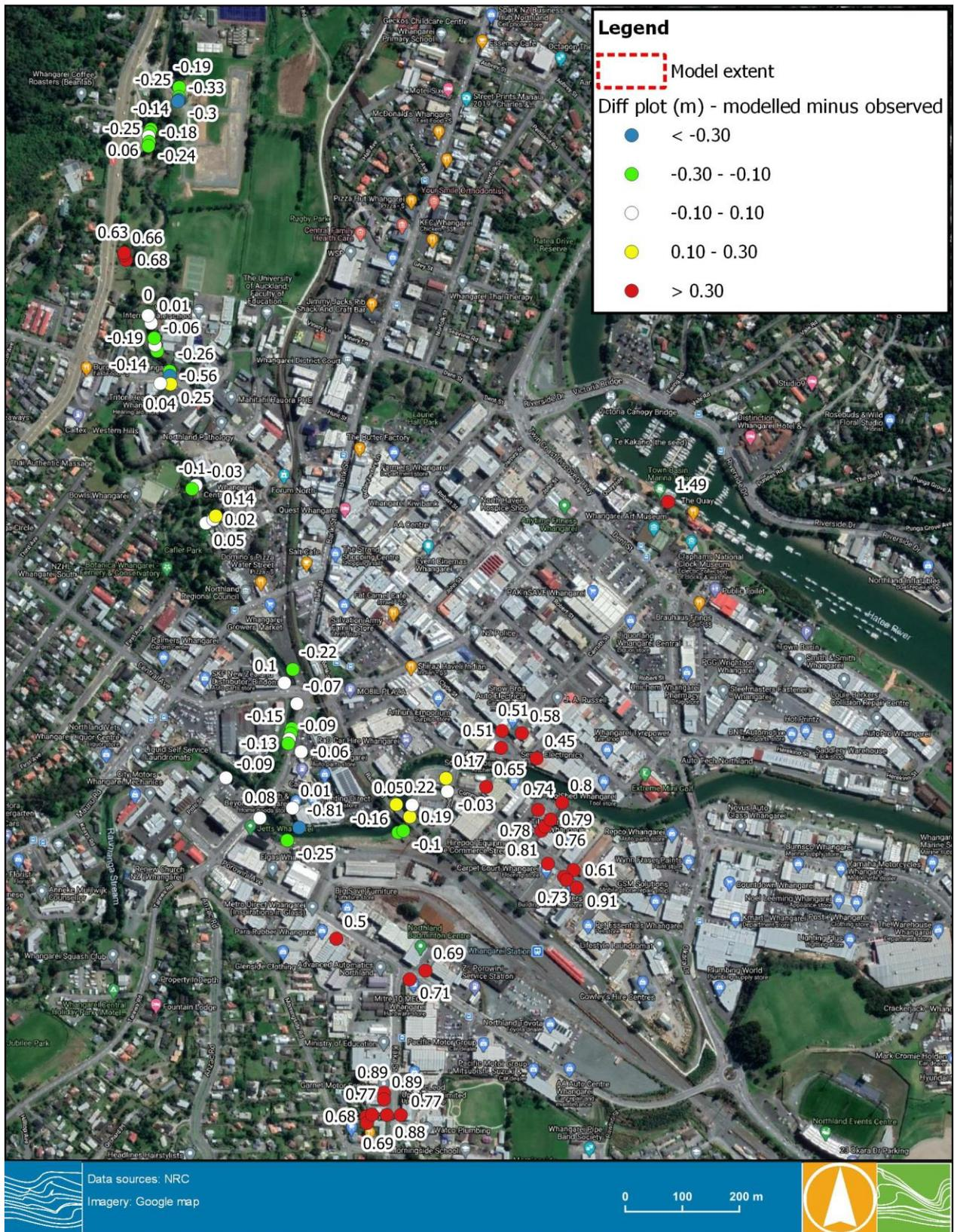
**FIGURE 6-20 COMPARISON BETWEEN MODELLED FLOOD LEVEL AND SURVEY FLOOD LEVEL – JANUARY 2011 EVENT (TOWNSHIP OF WHANGAREI)**
