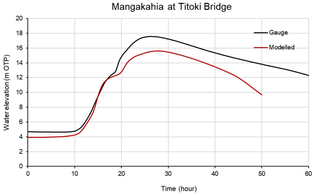
FIGURE 7-13 MODELLED AND GAUGED WATER LEVEL COMPARISON AT TITOKI GAUGE – M13
