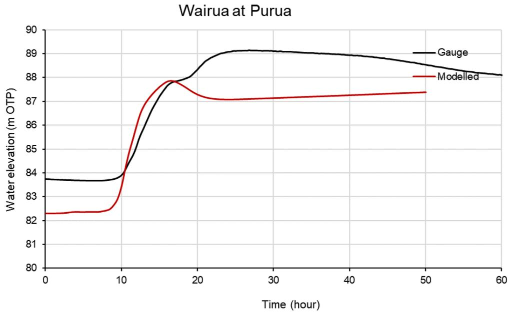
FIGURE 8-8 MODELLED AND GAUGED WATER LEVEL COMPARISON AT WAIRUA AT PURUA GAUGE – M14
