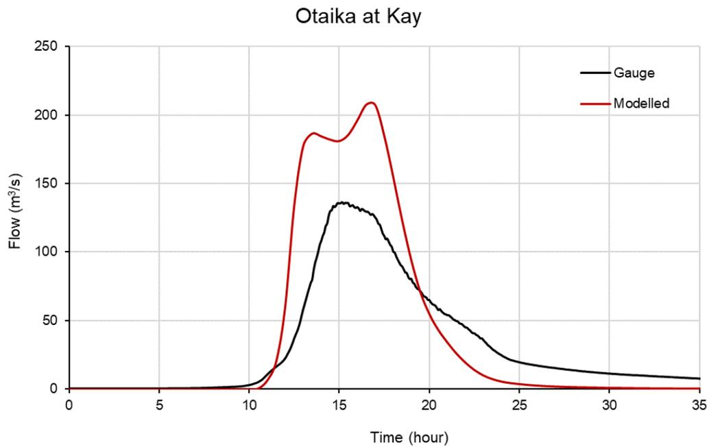
**FIGURE 6-13 MODELLED AND GAUGED FLOWS FOR OTAIIKA RIVER AT KAY – 2011 FLOOD EVENT**
