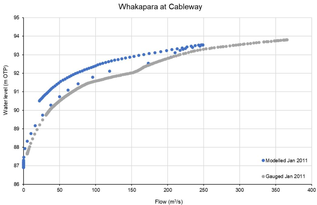
**FIGURE 8-13 MODELLED AND GAUGED RATING CURVE COMPARISON AT CABLEWAY GAUGE**
