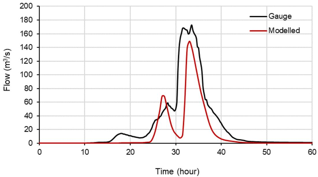
FIGURE 15-10 MODELLED AND GAUGED FLOWS AT TARAWHATORA RIVER AT SCHOOL CUT - JULY 2007 EVENT
