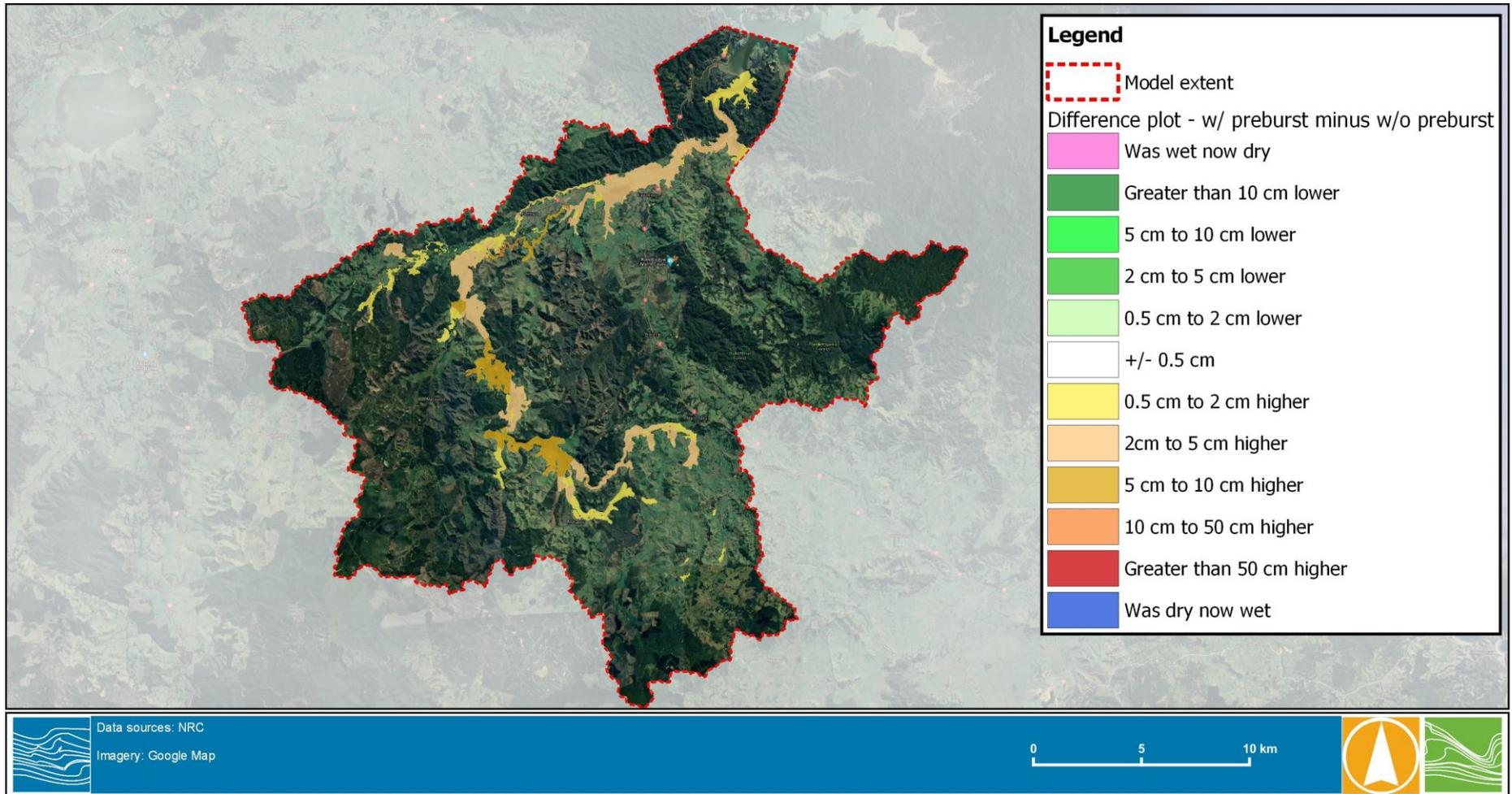
**FIGURE 9-9 DIFFERENCE PLOT OF PREBURST SENSITIVITY TEST IN KAWAKAWA CATCHMENT**
