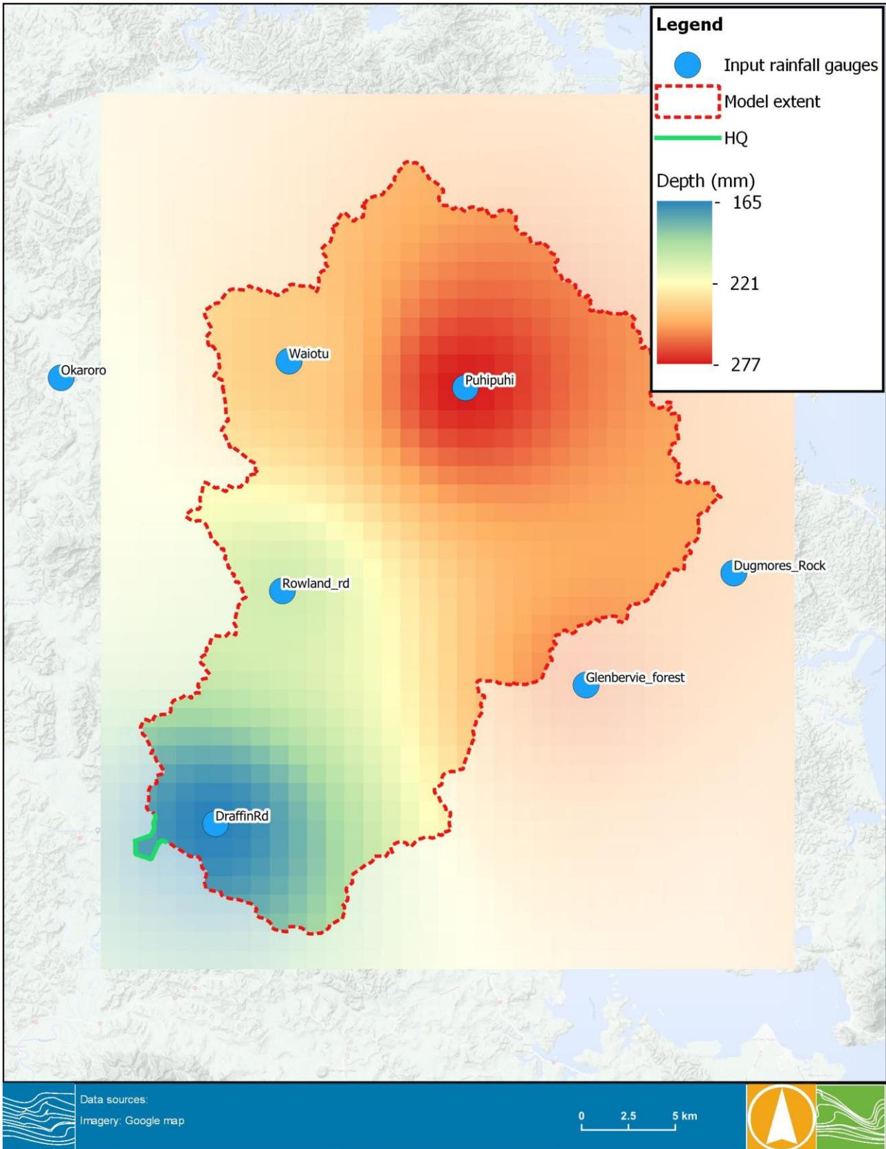
**FIGURE 8-3 HYDRAULIC MODEL BOUNDARIES AND INTERPOLATED RAINFALL DEPTH – M14**
