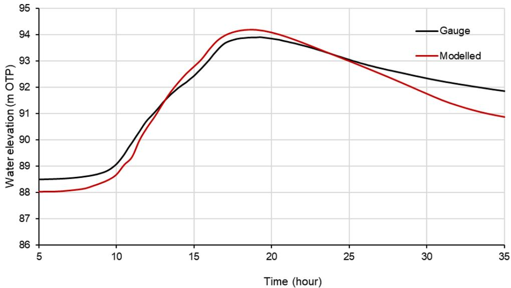
**FIGURE 8-5 MODELLED AND GAUGED WATER LEVEL COMPARISON AT S.H. 1 BRIDGE GAUGE – M14**
