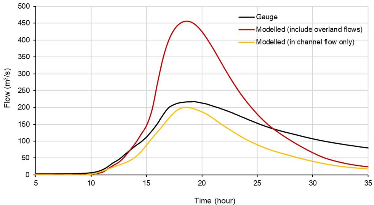
FIGURE 8-18 IN CHANNEL FLOWS AND OVERLAND FLOWS AT S.H.1 BRIDGE GAUGE
