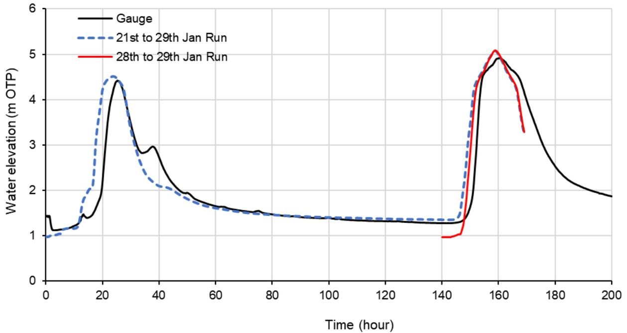
FIGURE 9-11 MODELLED WATER LEVEL HYDROGRAPHS FROM 21<sup>ST</sup> TO 29<sup>TH</sup> JANUARY RAINFALL – M06
