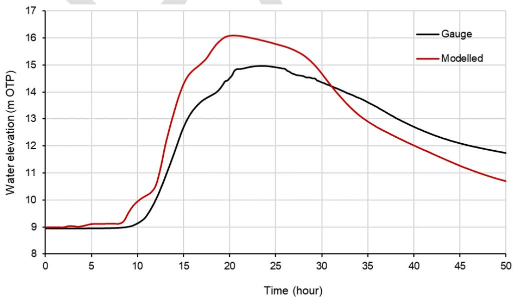
**FIGURE 15-5 MODELLED AND GAUGED WATER LEVELS AT AWANUI RIVER AT SCHOOL CUT – 2011 FLOOD EVENT**
