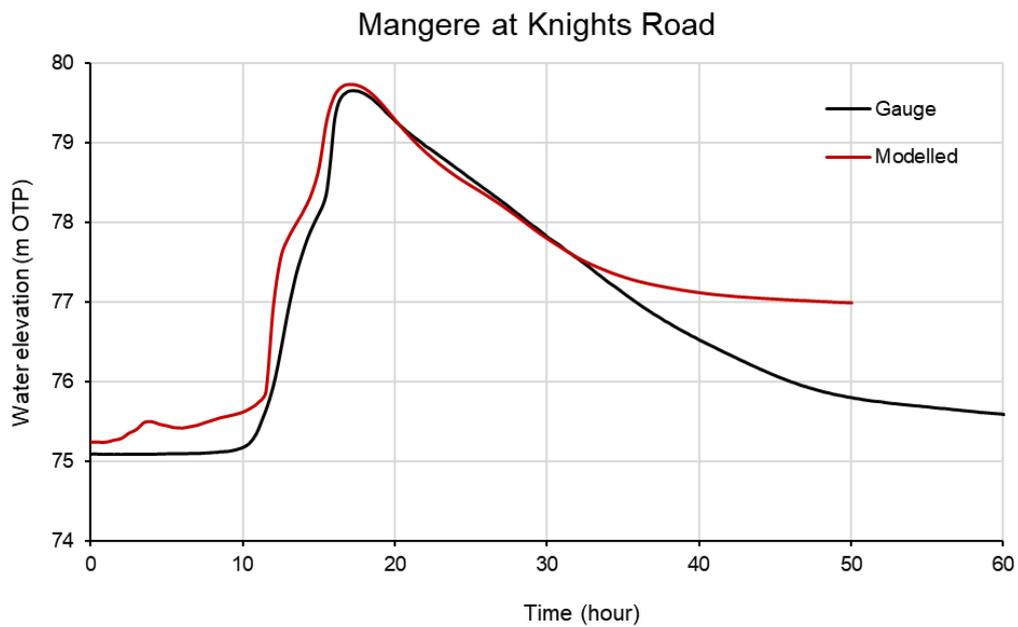
FIGURE 8-9 MODELLED AND GAUGED WATER LEVEL COMPARISON AT KNIGHTS RD GAUGE – M14
