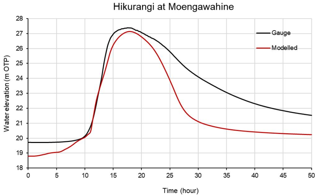
FIGURE 7-11 MODELLED AND GAUGED WATER LEVEL COMPARISON AT MOENGAWAHINE GAUGE – M13
