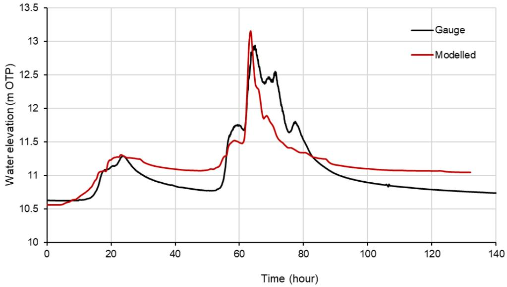
FIGURE 4-12 MODELLED AND GAUGED WATER LEVELS AT TARAWHATORA RIVER AT PURIRI PLACE – 2020 FLOOD EVENT
