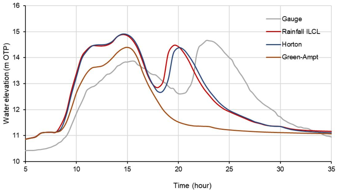
**FIGURE 9-4 WATER LEVEL COMPARISON OF DIFFERENT LOSS METHODS – TARAWHATAROA RIVER AT PURIRI PLACE**
