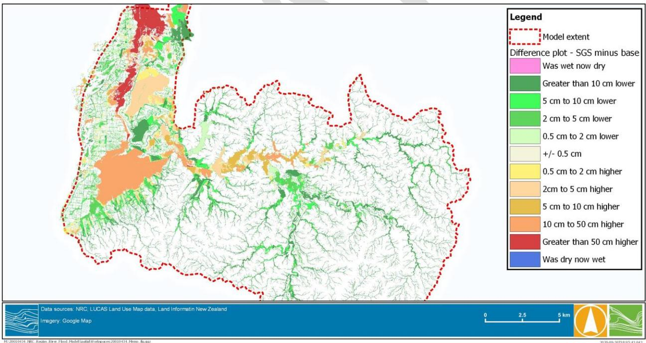
**FIGURE 3-4 FLOOD LEVEL DIFFERENCE PLOT (SGS AND BASE SCENARIO)**
