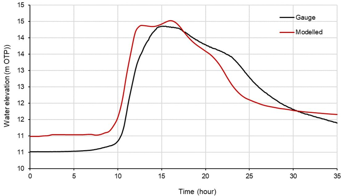
FIGURE 6-14 MODELLED AND GAUGED LEVELS AT OTAIIKA RIVER AT KAY – 2011 FLOOD EVENT
