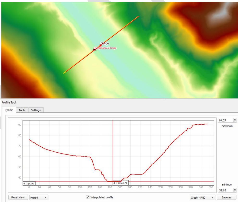
FIGURE 7-14 CHANNEL CROSS SECTION AT GORGE GAUGE
