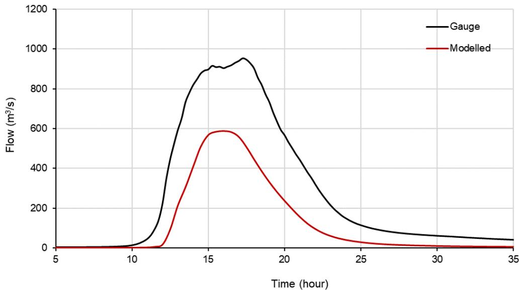
**FIGURE 7-6 MODELLED AND GAUGED HYDROGRAPH COMPARISON AT GORGE GAUGE – M13**
