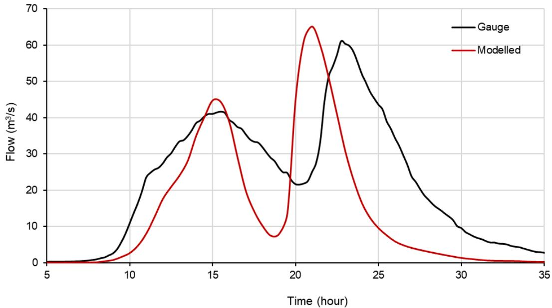
FIGURE 15-6 MODELLED AND GAUGED FLOWS AT TARAWHATORA RIVER AT SCHOOL CUT – 2011 FLOOD EVENT
