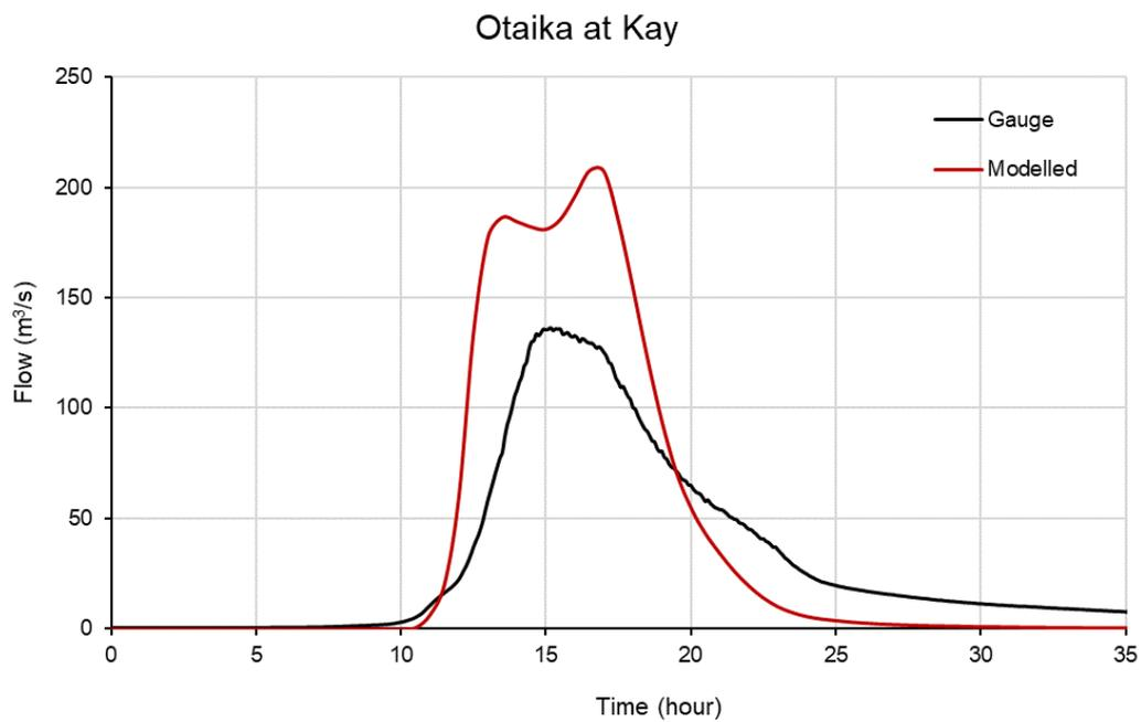
**FIGURE 3-7 MODELLED AND GAUGED FLOWS FOR OTAIIKA RIVER AT KAY – 2011 FLOOD EVENT**
