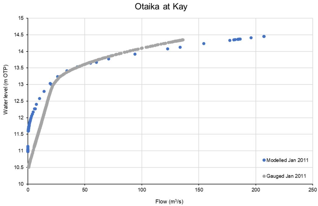
FIGURE 3-12 MODELLED AND GAUGED RATING CURVE COMPARISON AT KAY
