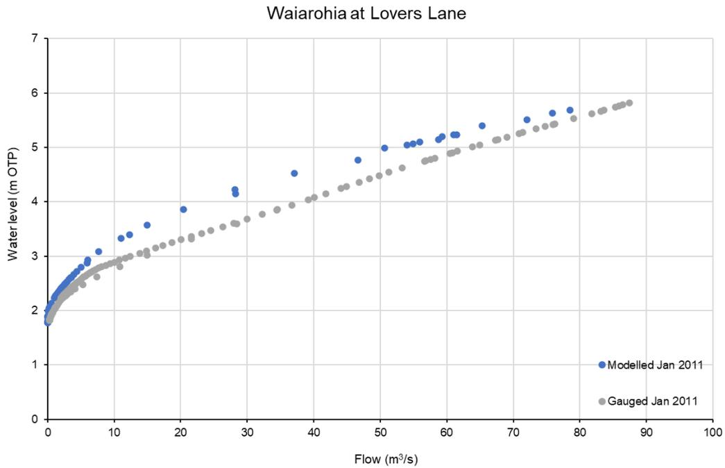
**FIGURE 3-10 MODELLED AND GAUGED RATING CURVE COMPARISON AT LOVERS LANE GAUGE**
