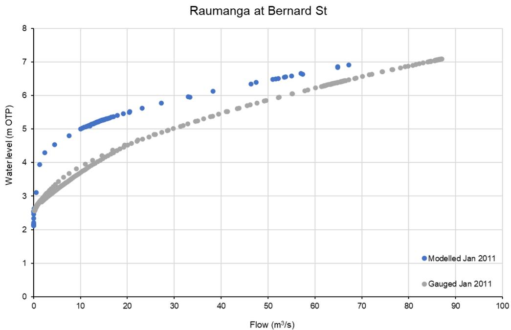
**FIGURE 3-11 MODELLED AND GAUGED RATING CURVE COMPARISON AT BERNARD ST**
