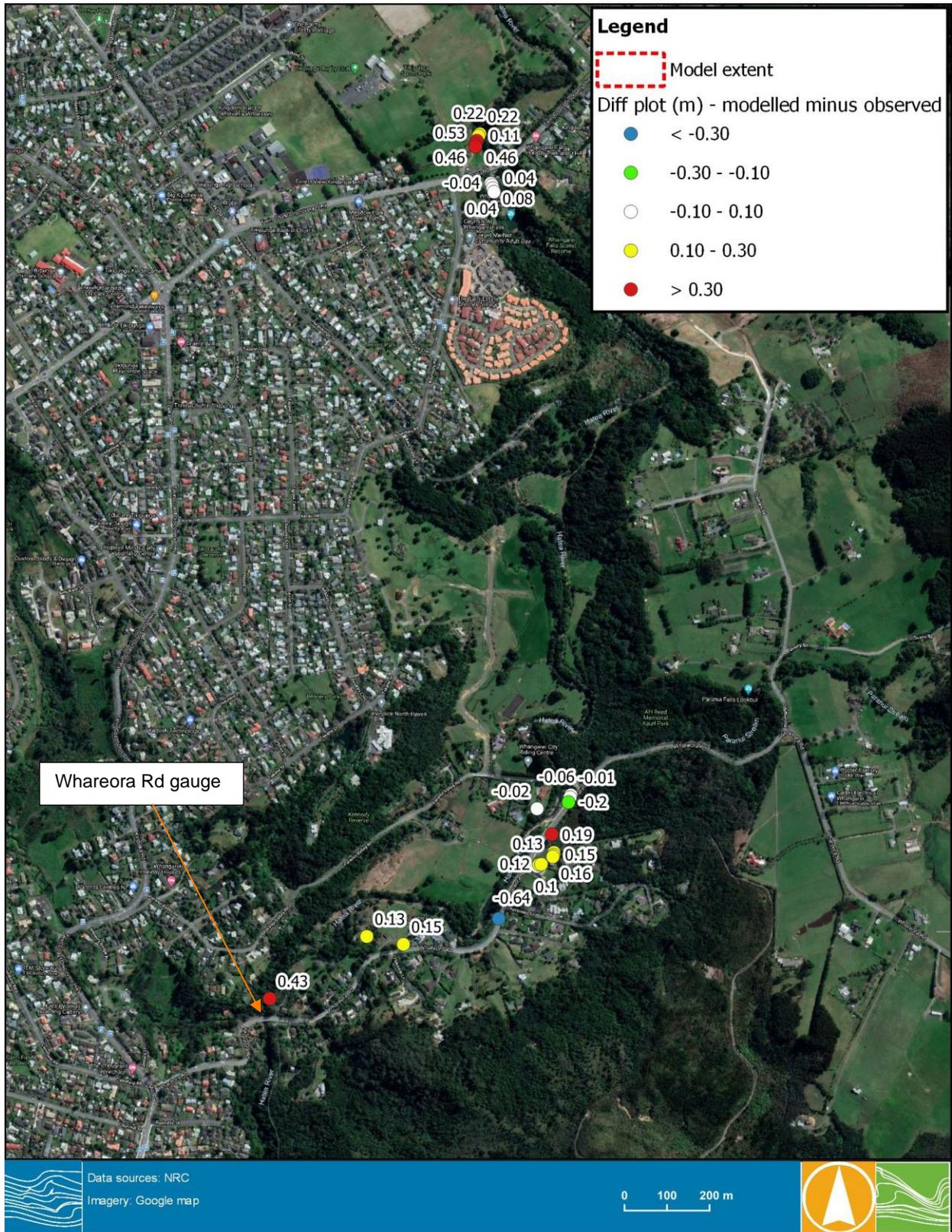
**FIGURE 3-13 COMPARISON BETWEEN MODELLED FLOOD LEVEL AND SURVEY FLOOD LEVEL – JANUARY 2011 EVENT (UPSTREAM OF WHAREORA RD GAUGE)**
