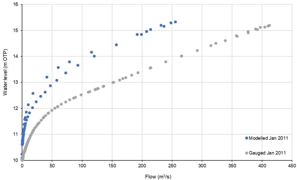
FIGURE 3-9 MODELLED AND GAUGED RATING CURVE COMPARISON AT WHAREORA RD GAUGE
