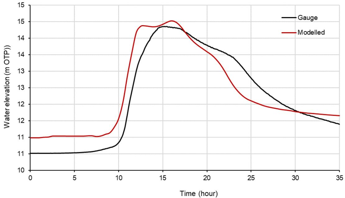
FIGURE 3-8 MODELLED AND GAUGED LEVELS AT OTAIKA RIVER AT KAY – 2011 FLOOD EVENT
