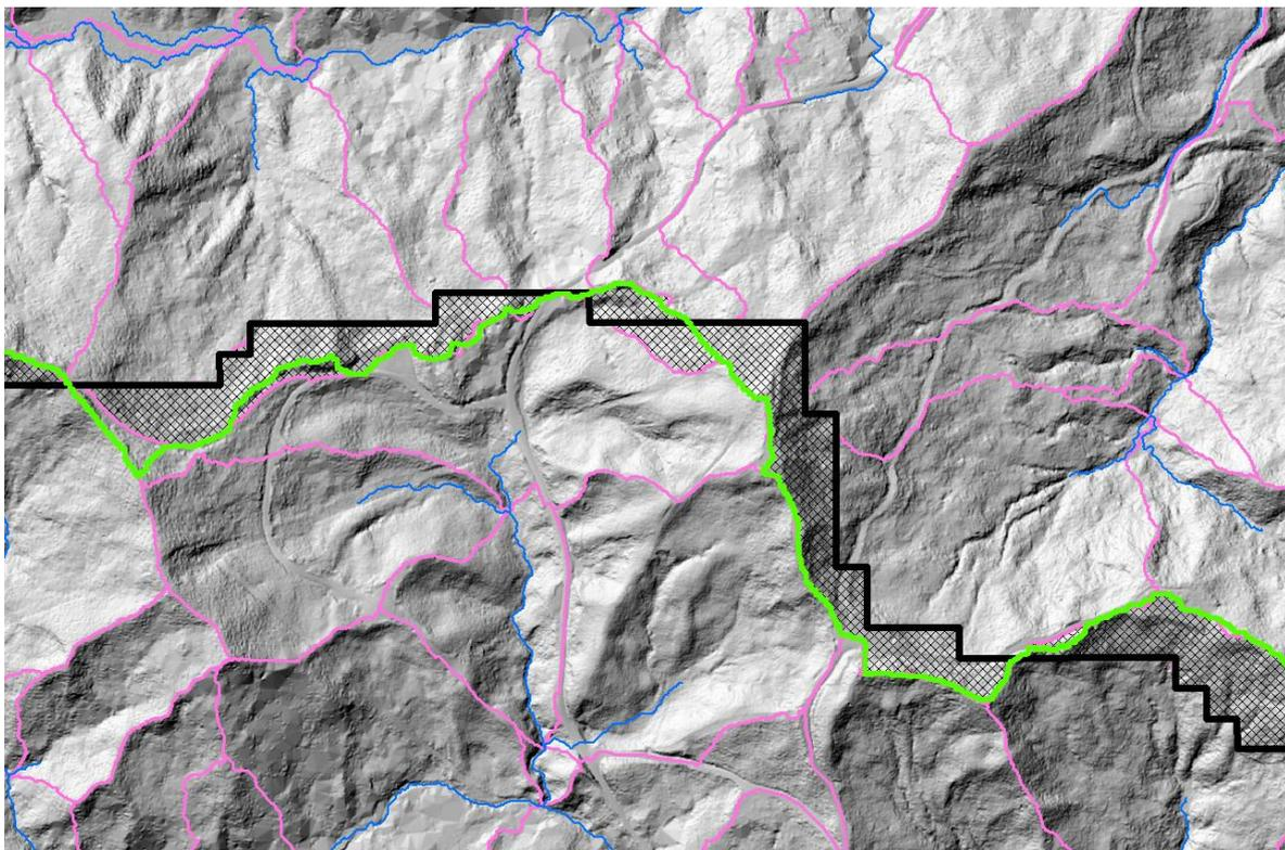
**Figure 3-2** The discrepancy of catchment areas (black hatched areas) between the NRC FMU boundary (thick black line) and the improved FMU boundaries (green line) using NRC LiDAR.
