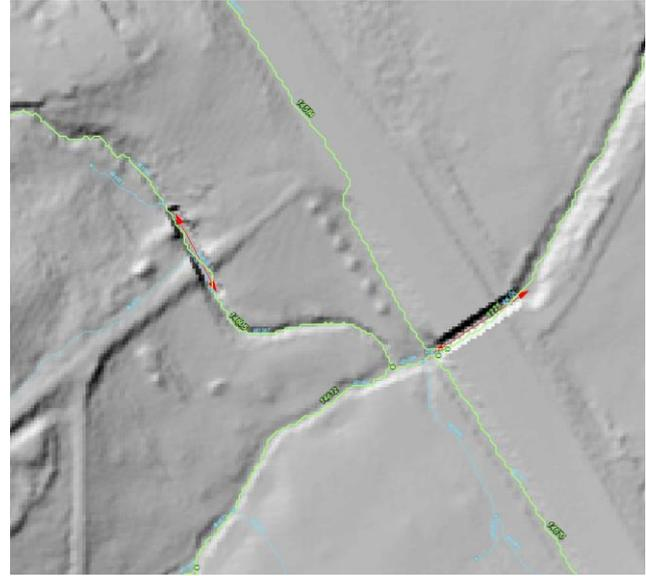
**Figure 2-3** Burnt culverts and resulting DRN
