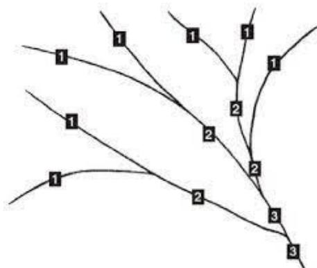
**Figure 5-1** Strahler stream order methodology
