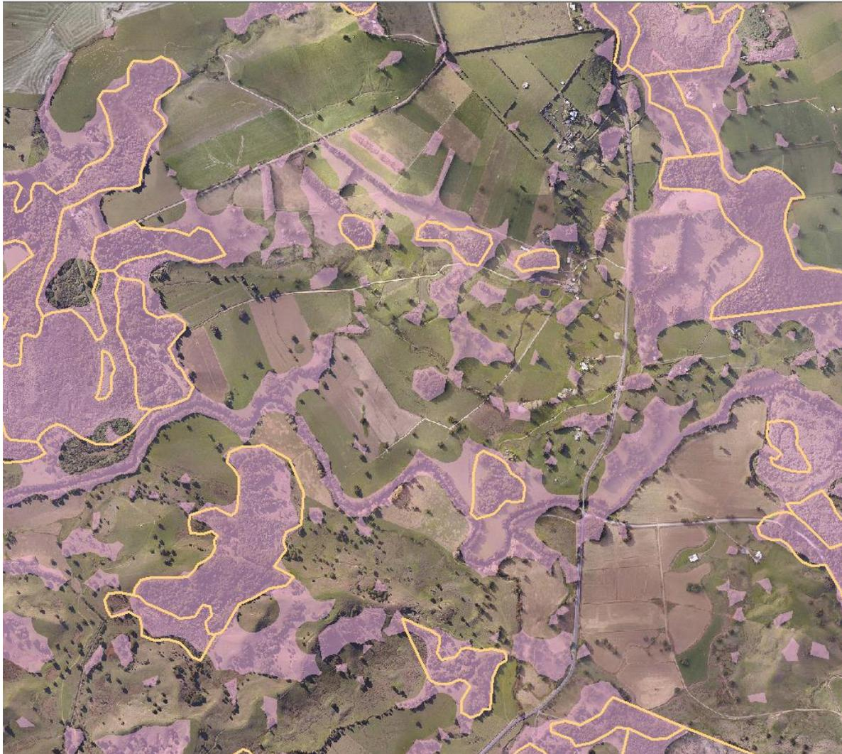
**Figure 5-7** New woody vegetation map based on Sentinel-2 (10m spatial resolution) satellite image classification compared to LINZ vegetation polygons (polygons in orange outlines).
