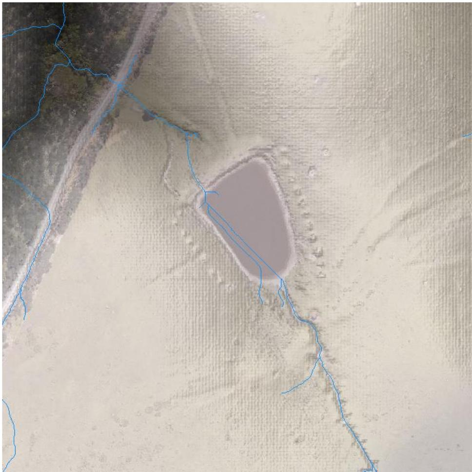
**Figure 7-2** Example of a drainage line through an 'un-burnt' farm dam, with minimal deviation in the overall drainage line on the upstream or downstream side of the dam
