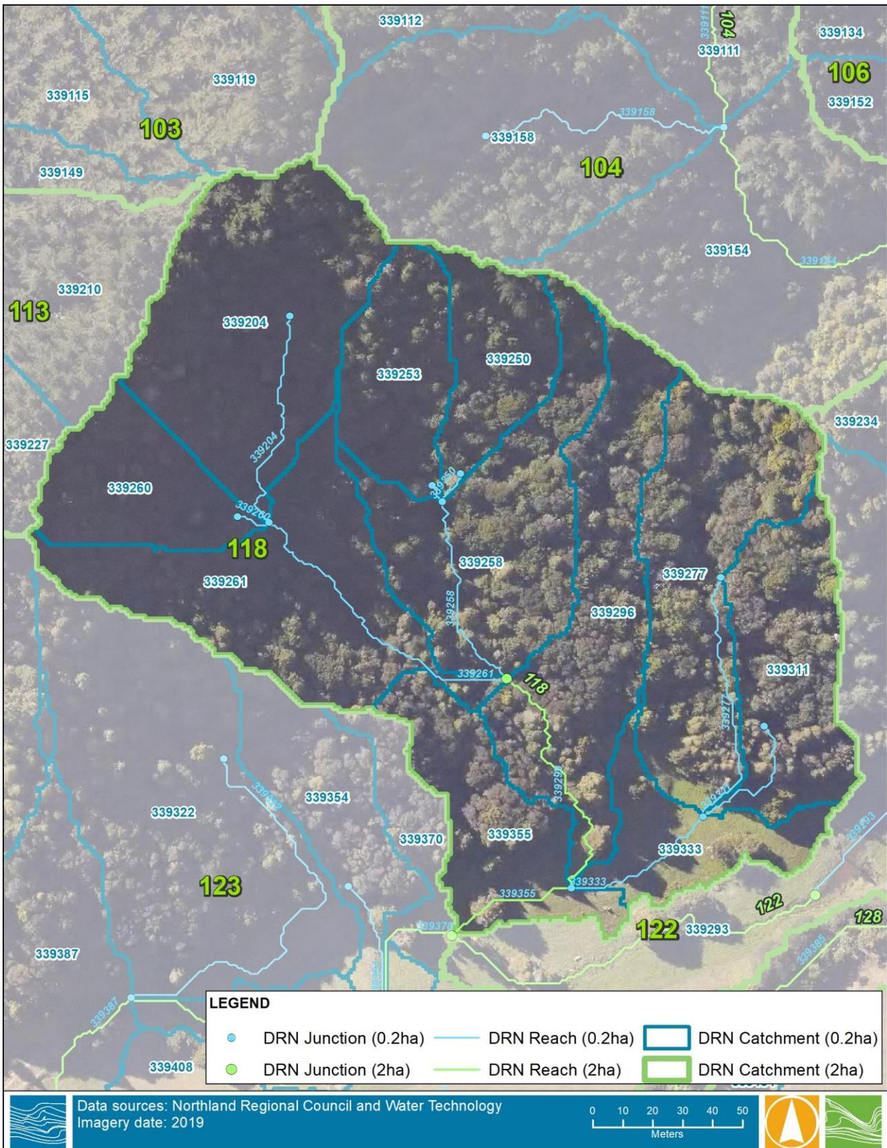
**Figure 4-3** Example of the final spatial outputs (vector dataset) for the Northland DRN model.
