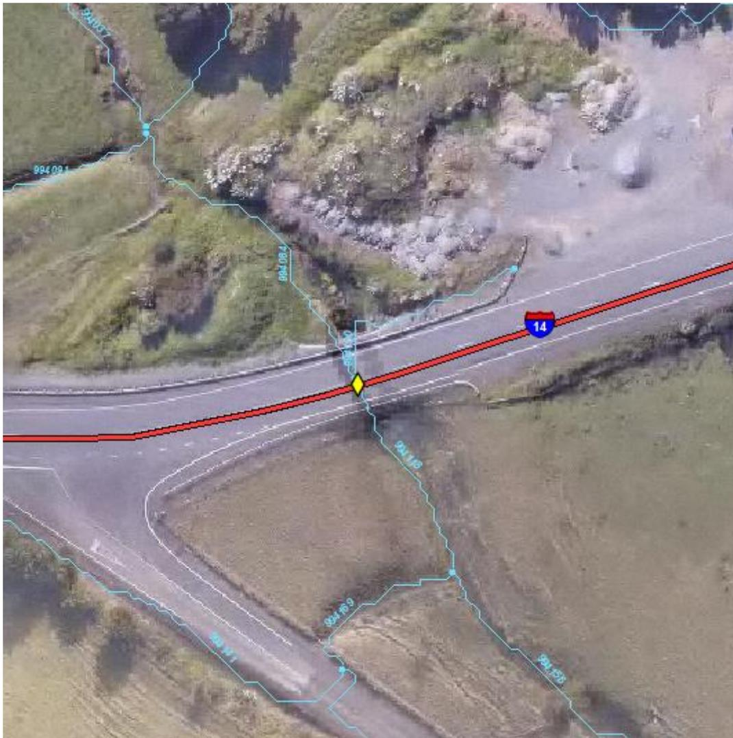
**Figure 4-4** Example stream crossing point representing potential fish passage barrier.
