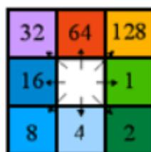
**Figure 4-1** D8 flow direction raster values
