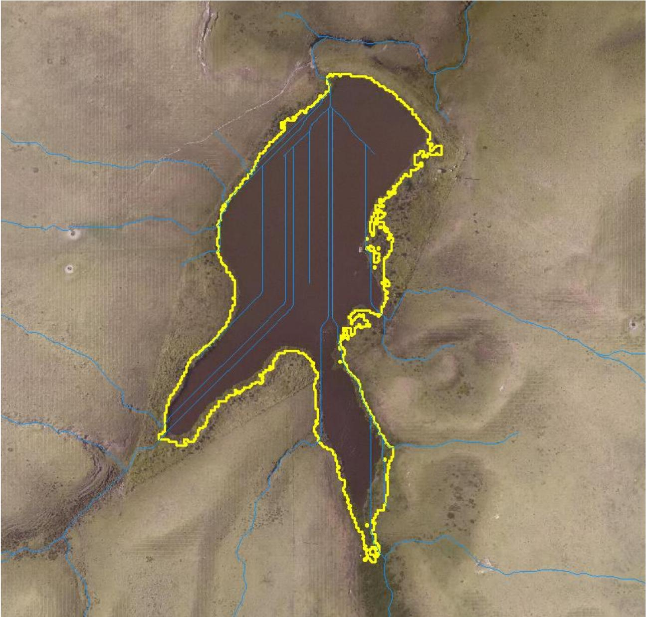
**Figure 7-3** Example of a lake with no burn line created – the drainage lines within the lake are not accurate, but the inflow and outflow drainage lines remain accurate
