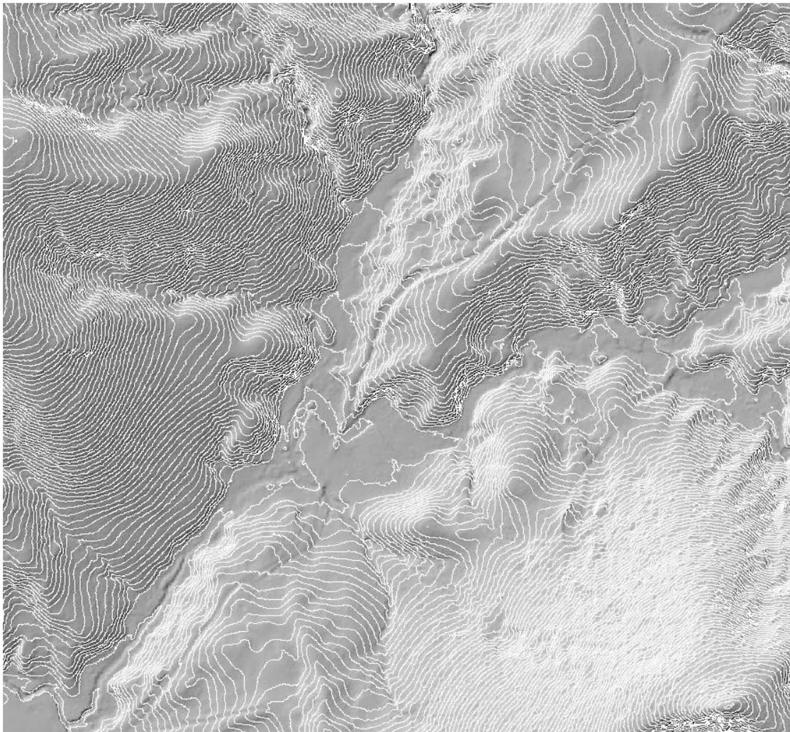
**Figure 4-5** An example of ‘hillshade’ version of the HE-DEM and 1m contours
